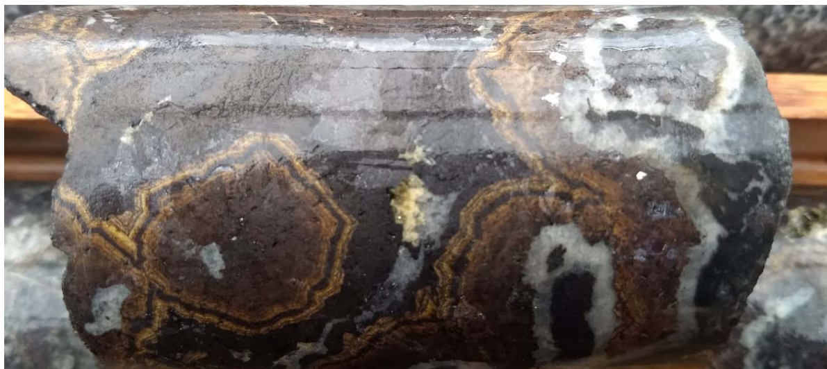
Figure 3. Detailed photo of zinc sulphide textures (see arrow above): iron rich sphalerite or marmatite (purple) with bands of later low iron sphalerite (brown and yellow) and quartz (white). The banding of the zinc sulphides highlights multiple stages of zinc mineralization at Ayawilca.
