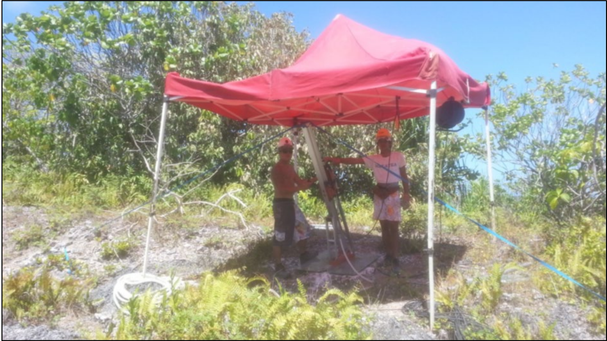
Figure 21: Hilti 350 drill assembly (Sawyer, 2014).
