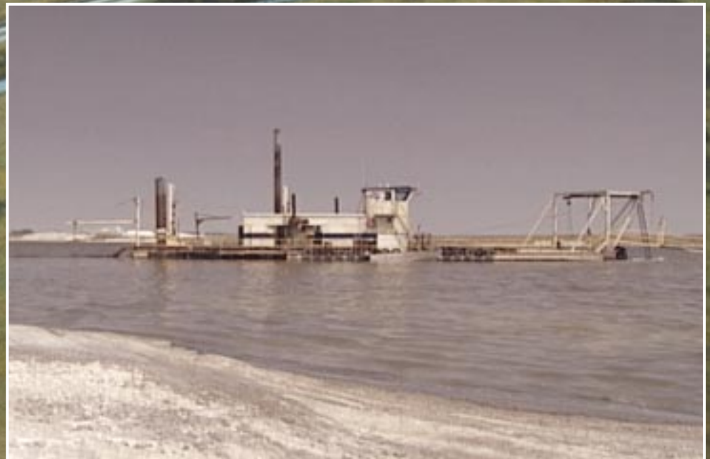
Sodium sulphate at the Ingebrigt facility is recovered from the salt deposit located under a 700 acre lake, by use of a floating dredge, equipped with a cutting head.
