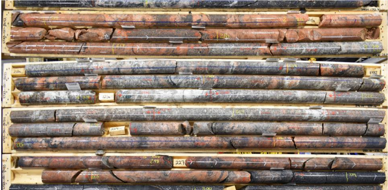
Figure 2: LT-23-21 Spodumene bearing pegmatite, 213.9 m – 228.75 m
