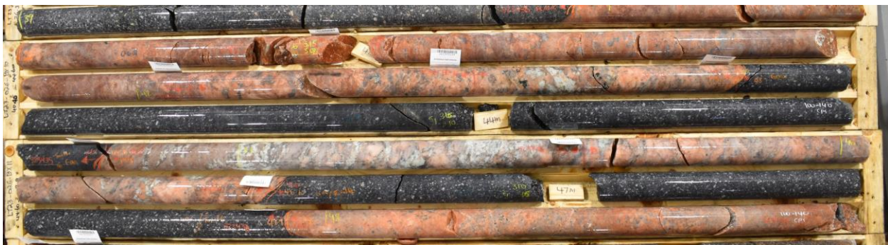
Figure 1: LT-23-26 Spodumene bearing pegmatite intercept, 39.9 m - 49.0 m
