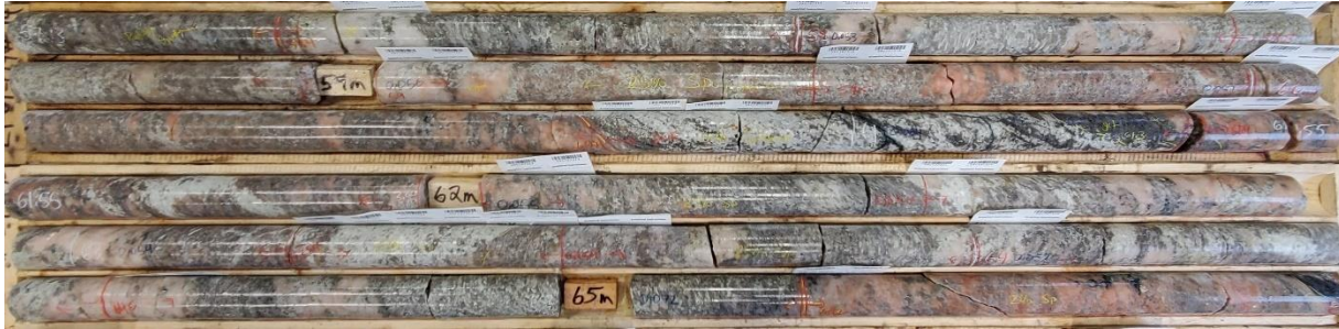
Figure 5: Mineralized (spodumene) Eagle Pegmatite intercept from drill hole LT-21-09
