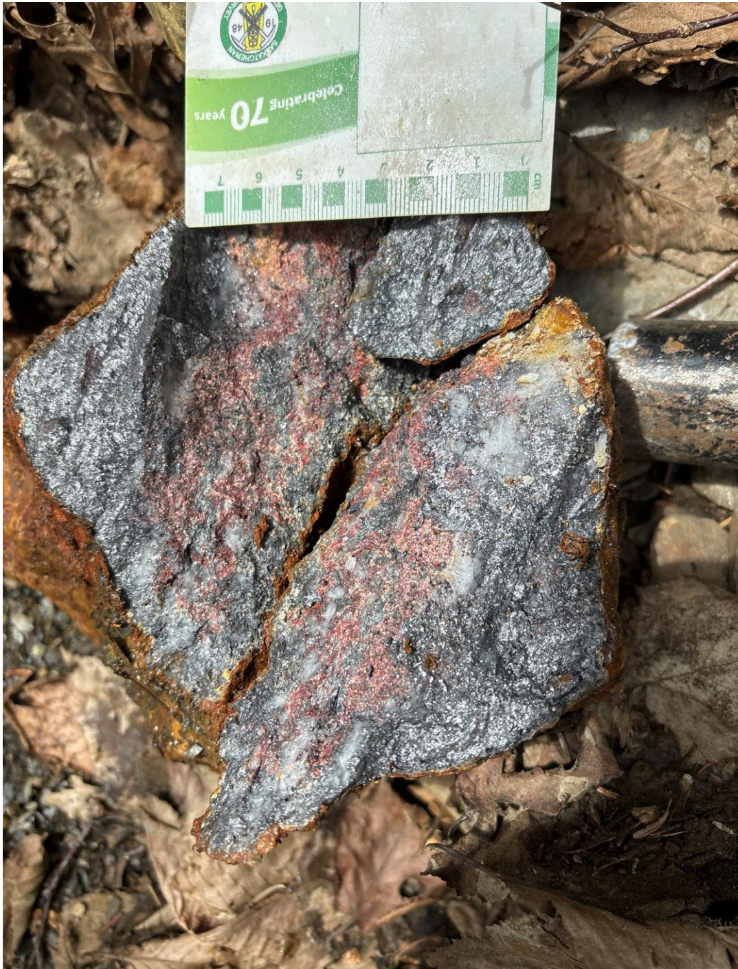
Figure 3C. Massive stibnite-quartz-kermesite float sample from southeast of Antimony Ridge.
