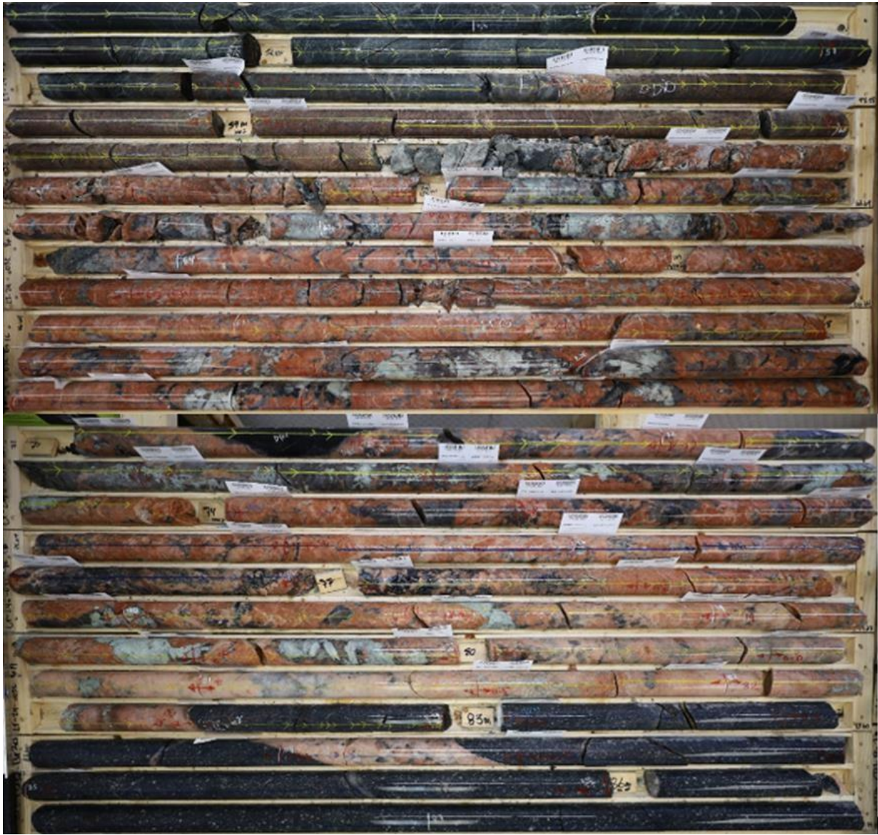
Figure 7. Drill Hole LT24-032 showing FD5 pegmatite hosting pale green spodumene blades intercept from 60.80 - 82.55 meters (assay results pending)
