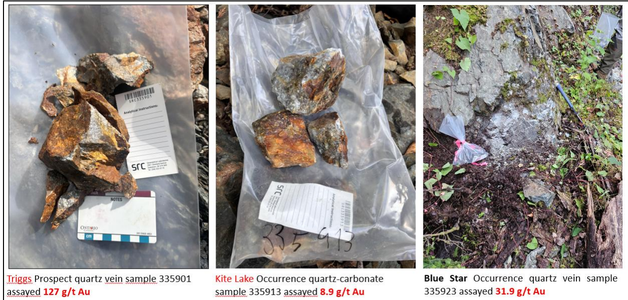
Figure 2. Photographs of Selected Due Diligence High-Grade Samples Collected by NAM Technical Representatives
