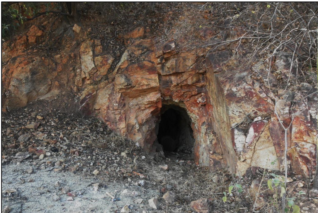
Figure 4. Sampling (channel 0.3 metres) to right of 1.5metre wide adit, silicified breccia, N30°E fracturing filled with quartz and sulphides, El Chon artisanal workings on Diamante 1.
