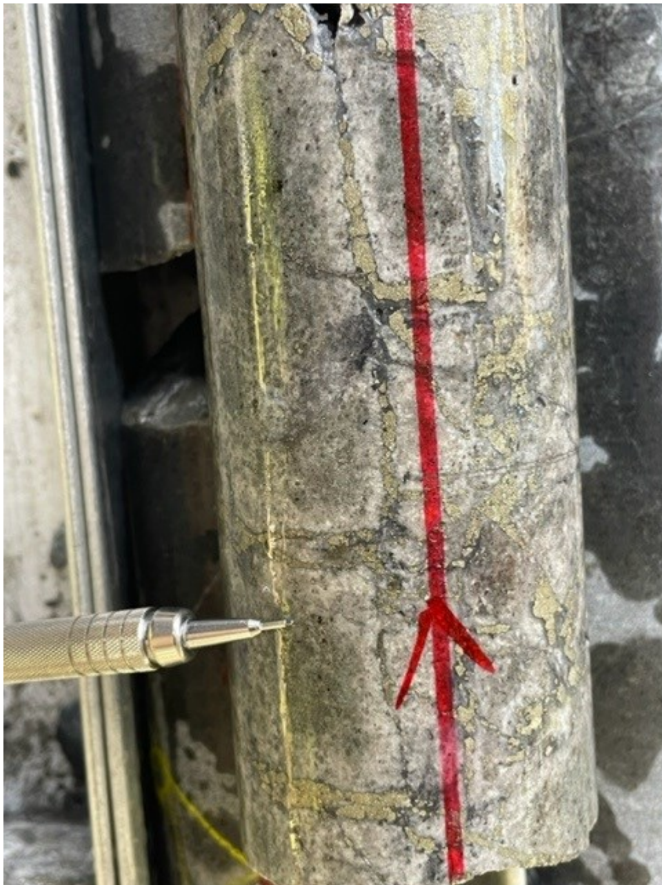
Figure 9: TUDDH 608. High-grade material hosted within mm-scale ladder vein at 606.5m. Grade: 54.54 g/t Au
