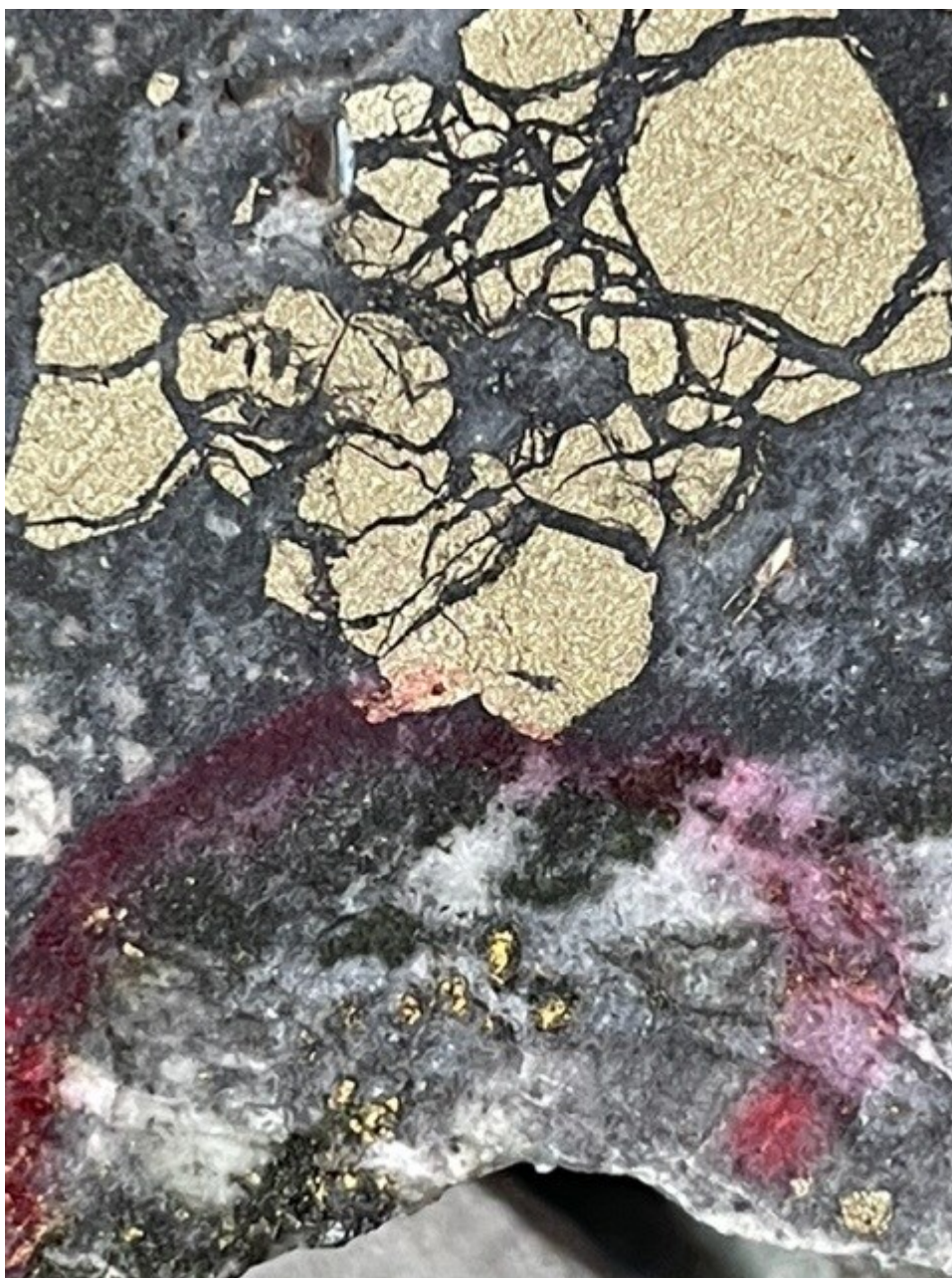
Figure 10: TUDDH 608. Visible gold in cut core. Grade: 45.02 g/t Au
