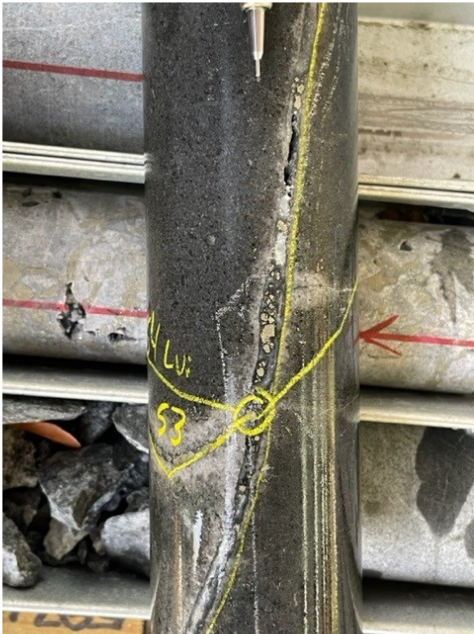
Figure 7: TUDDH 608. Gold-bearing mm-scale veins at 600.8m. Grade: 13.54 g/t Au
