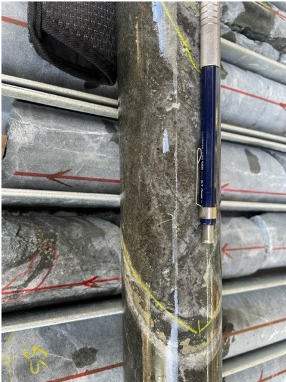
Figure 6: TUDDH 608. Gold-bearing veins at 600.5m. Grade: 21.69 g/t Au
