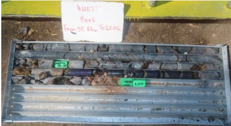
Figure 1 : Shaft #1 Drill Core from Level 1 Sub-level 1 – KWO-239 — Figure 1 shows massive bornite adjacent to a stope at the end of hole (KWO239).
