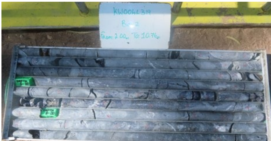
Figure 2: Shaft #1 Drill Core from Level 3 Sub-level 1 – KWO-256 — Figure 2 shows bornite and chalcopyrite occurring in highly calcified and fractured zone
