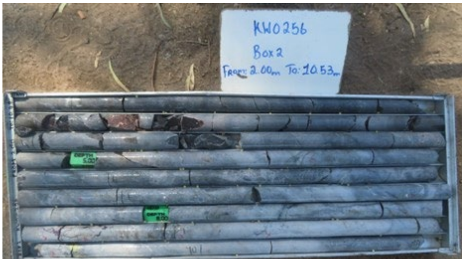
Figure 2: Shaft #1 Drill Core from Level 3 Sub-level 1 – KWO-256 — Figure 2 shows bornite and chalcopyrite occurring in highly calcified and fractured zone
