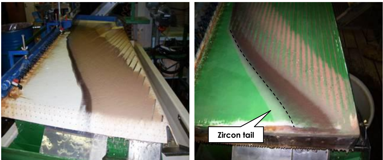
Figure 5: Rougher stage (left) and Cleaner stage (right) gravity separation of HM undertaken by Mineral Technologies Pty Ltd on bulk sample from the Argo prospect. Source: Combined Annual Report (C96/2003 Mt Jowlaenga) for the Period 21 July 2007 to 20 July 2008 Rio Tinto Exploration Pty Ltd.
