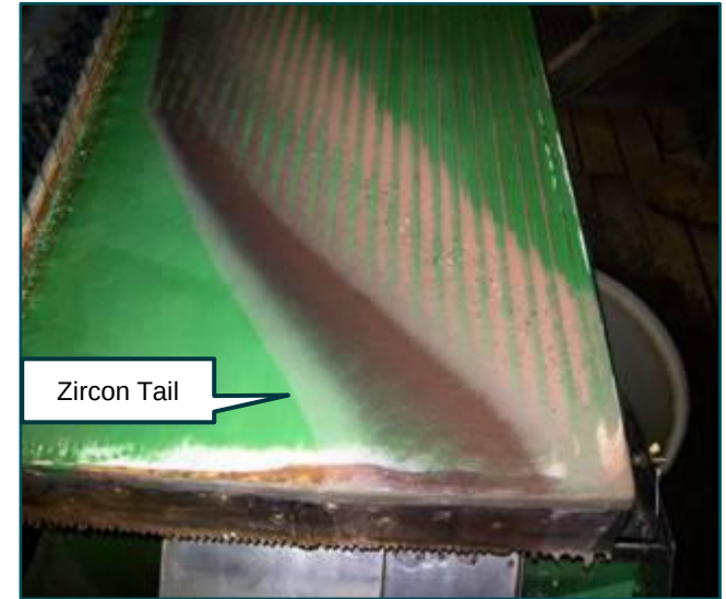
Cleaner stage gravity separation of HM on bulk sample from the Argo prospect. Source: Rio Tinto Exploration Pty Ltd open file report.
