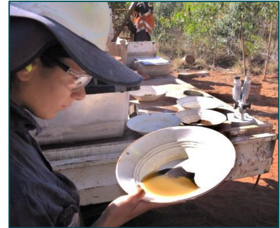
Panning of heavy mineral from drill sample
