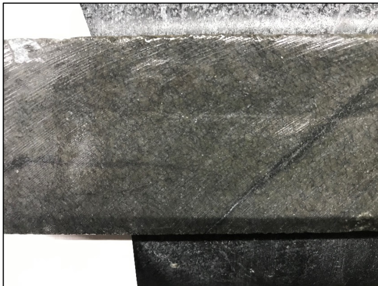
Photo 9: Cumulate texture of the dunite as observed in drill core. Green olivine grains are rimmed by magnetite (black).
