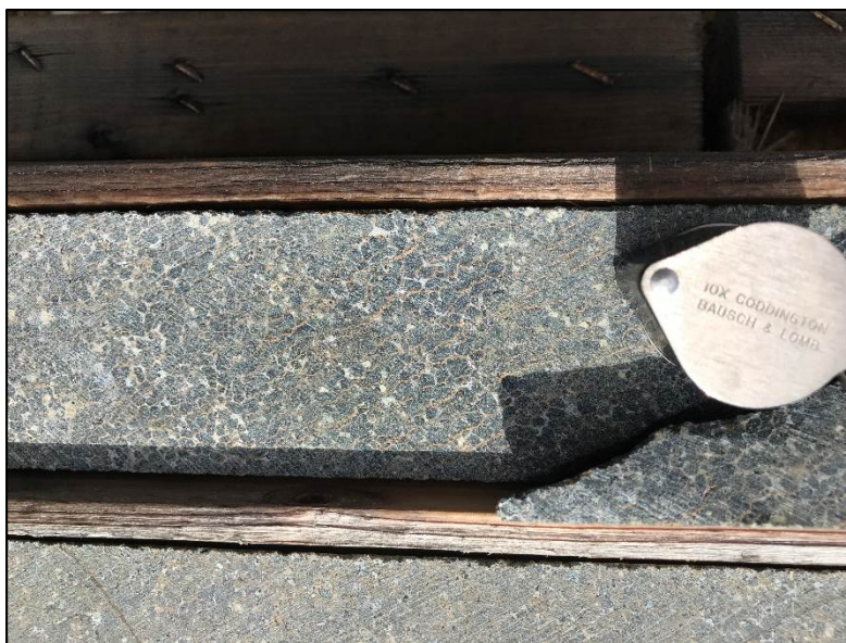
Photo 10: Cumulate texture of slightly weathered dunite. Weathering as a result of the core lying outdoors. Sample comes from a depth of about 190 m in hole CRAW18-02.
