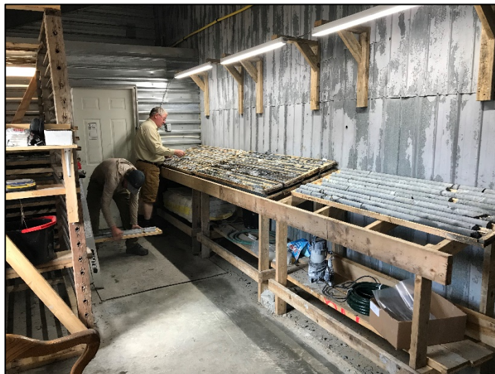
Photo 6: Logging and sampling facility in Timmins, Ontario. Core saw for splitting the logged core is located in the room at the rear of the core shack.
