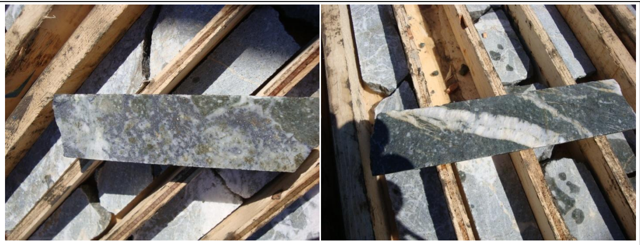
Figure 8-1. Silver Coin Project - Right, Low Sulphide Mineralisation with Quartz Veining. Left High Sulphide Mineralisation with Silicification.
