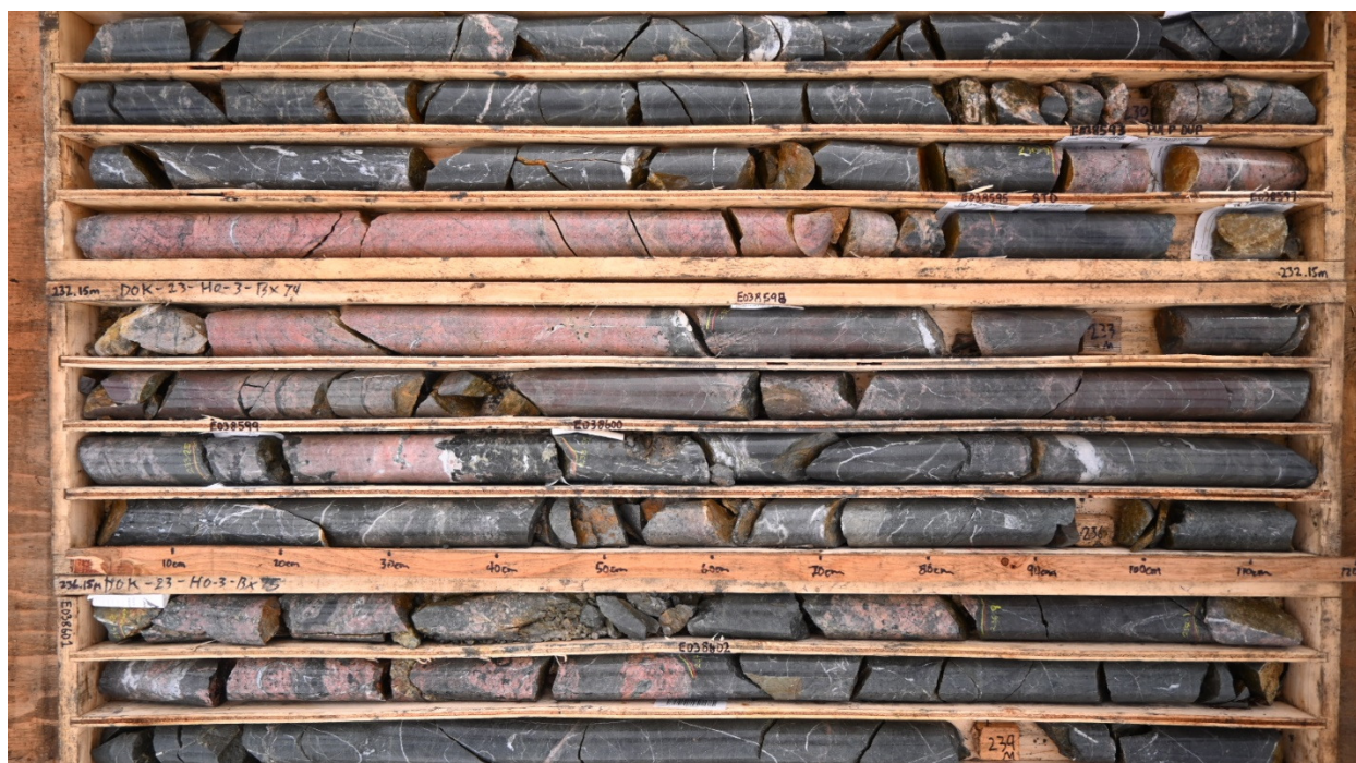
Figure 3 - DK2023-03 from 229.1 to 237.7 meters yielding 8.6 meters of 0.57 Cu Eq (%).
