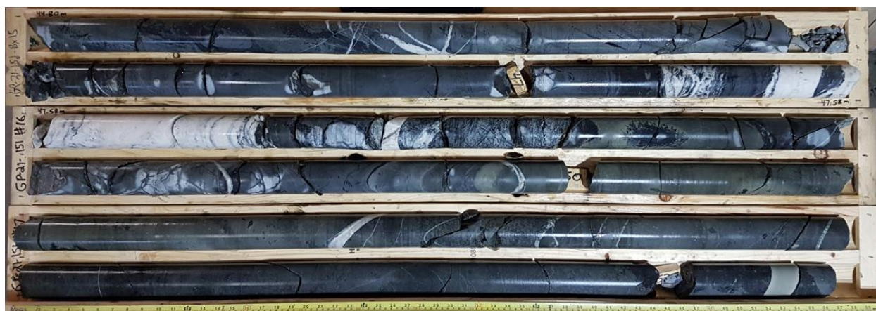
Quartz Veined Interval in GP-21-151 with Visible Gold
