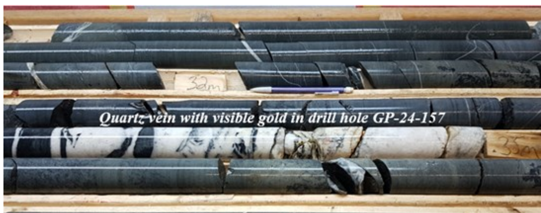
Quartz vein with visible gold in drill hole GP-24-157 (JMZ - Golden Promise Gold Property)
