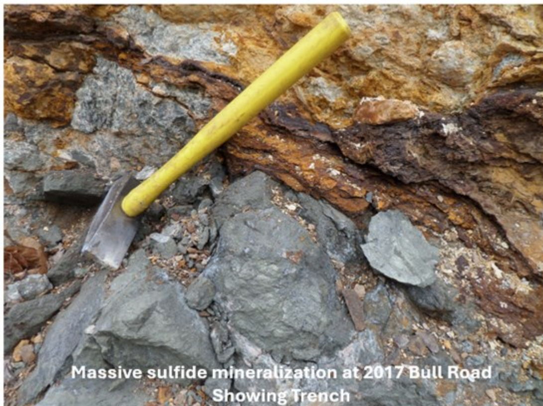
Massive sulfide mineralization at 2017 Bull Road Showing Trench
