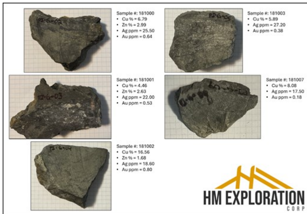
Figure 1: Outcrop samples collected at the Zone in 2025 displayed impressive mineralization including both massive and disseminated chalcopyrite ± sphalerite, silver, gold, and lead*.
