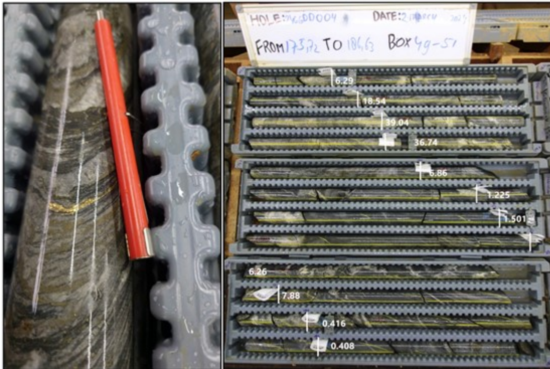
Figure 3: (left) gold vein in drill core from hole 24GG04. (right) Drill core from hole 24GG04 showing typical textures within mineralized zones at Froyo. Core locally contains up to 35% pyrrhotite and pyrite within a zone of high-intensity shearing.
