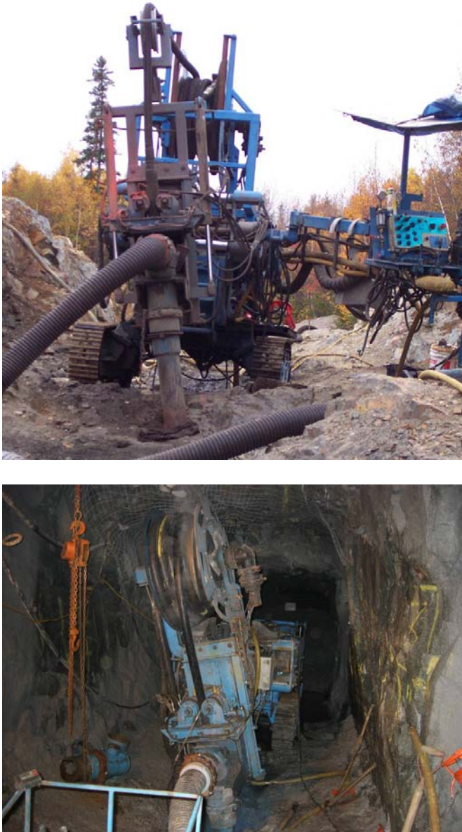
Figure 36 : Thermal fragmentation drill in action on surface and underground
