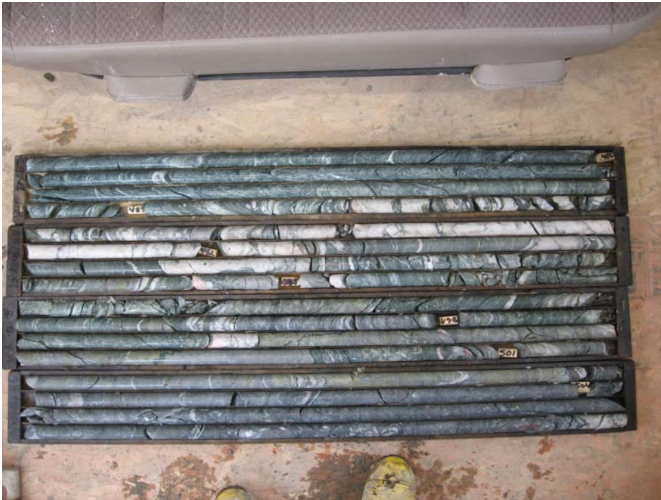
Figure 5: Picture of the core - Boucher zone at 490m
