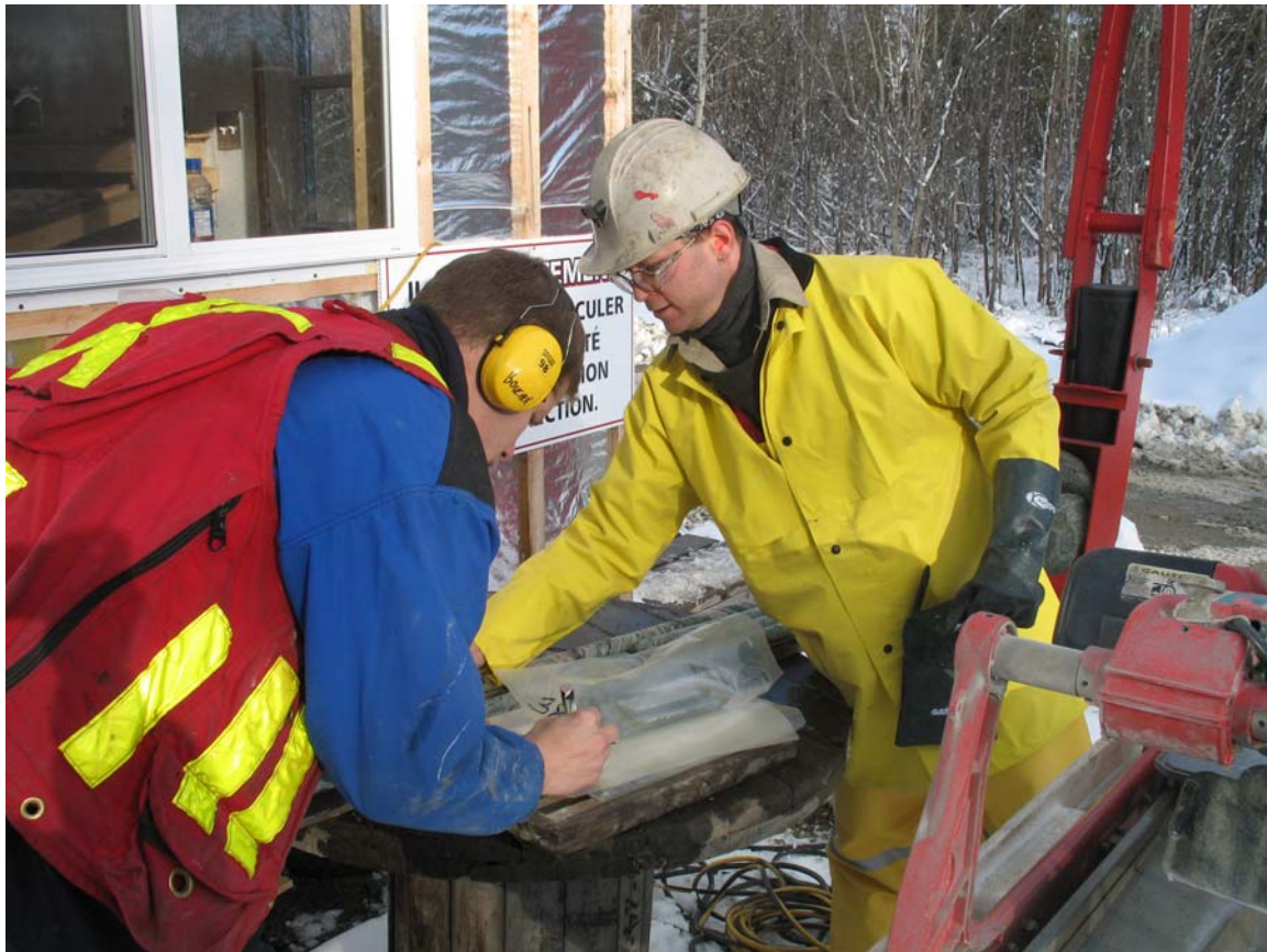
Figure 11: Sawing of core and sampling at Rocmec 1 outside core shack
