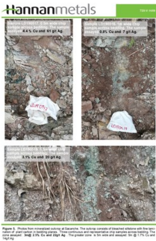
Figure 5. Photos from mineralized outcrop at Sacanche. The outcrop consists of bleached siltstone with fine lamination of plant carbon in bedding planes. Three continuous and representative chip samples across bedding. The zone assayed: 3m @ 2.5% Cu and 22 g/t Ag. The greater zone is 5m wide and assayed: 5m @ 1.7% Cu and 14 g/t Ag (CNW Group/Hannan Metals Ltd.)
