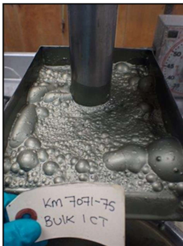
Figure 1. Bulk concentrate during cleaner test, demonstrating froth quality.
