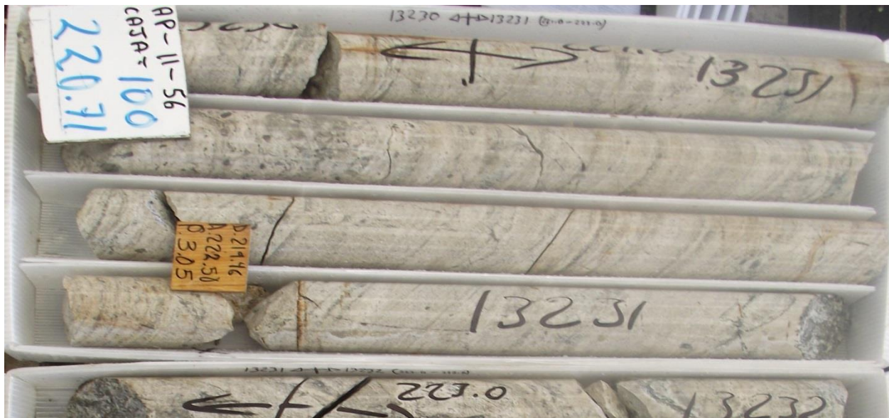
Figure 7-8: Banded Fine Grained Intrusive Phase, Intrusive Domain
