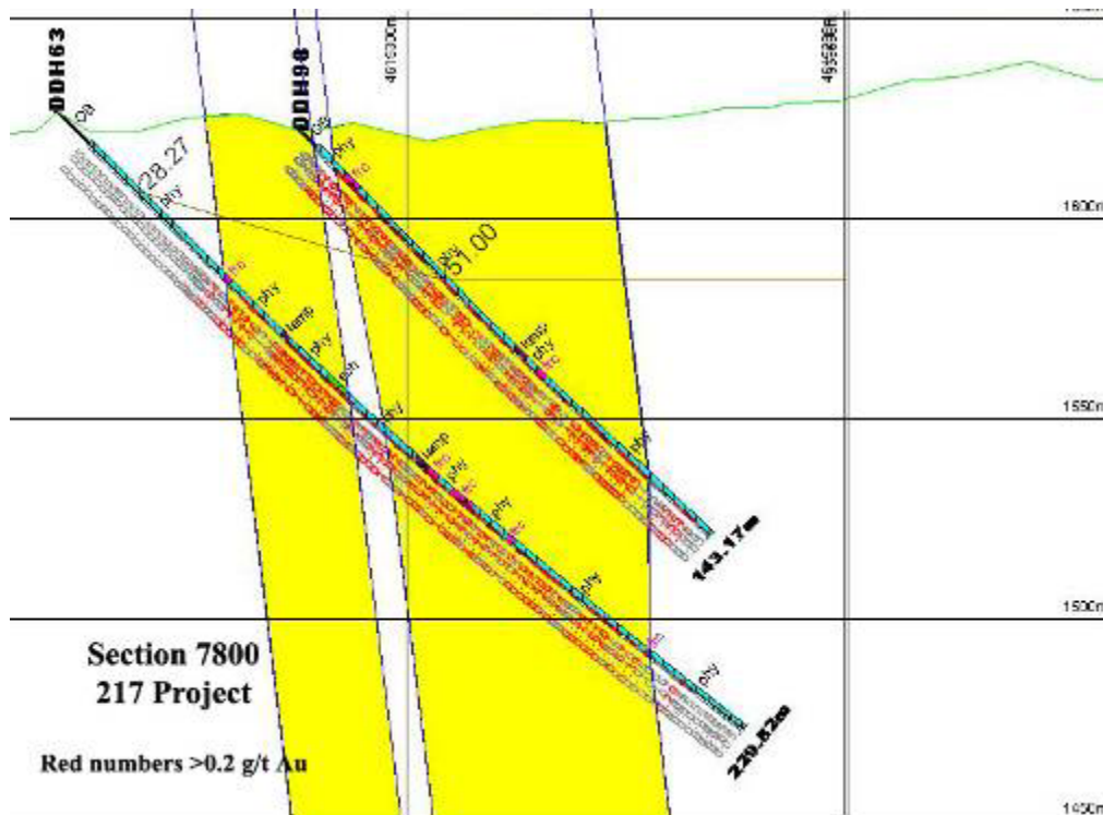
Figure C.8: Interpreted Section 7800 showing drill hole data, interpreted 0.20g/t zone, oxide/sulphide interface, and topography.
