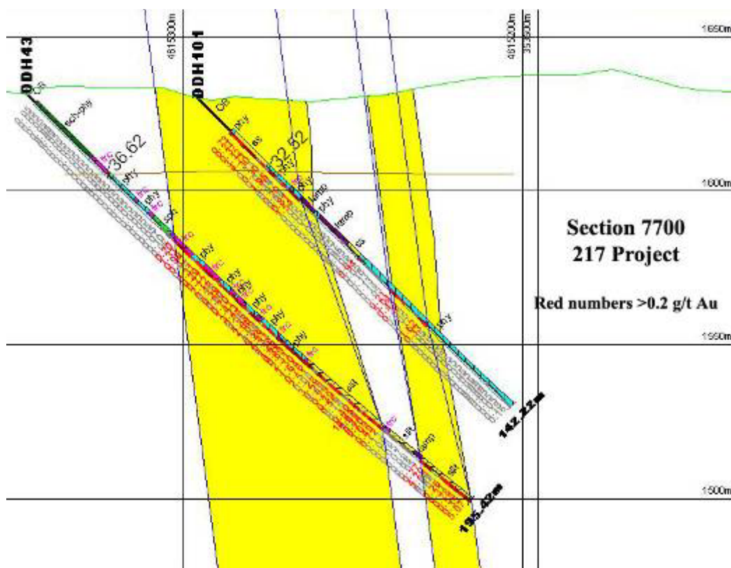
Figure C.6: Interpreted Section 7700 showing drill hole data, interpreted 0.20g/t zone, oxide/sulphide interface, and topography.
