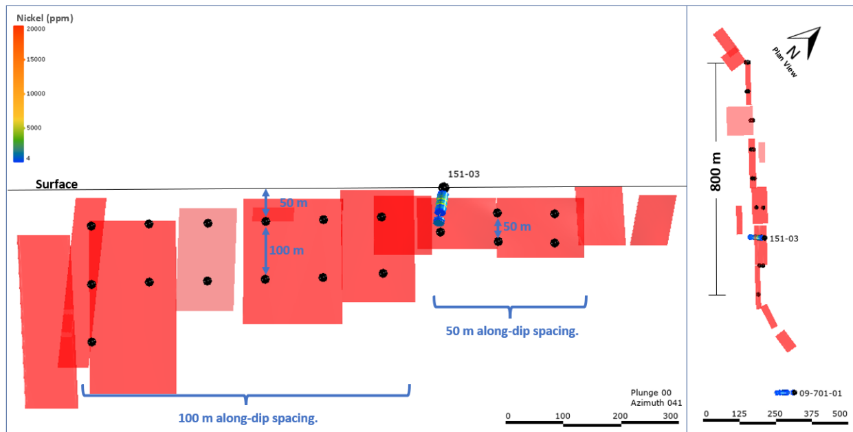
Figure 4 - Long-section view looking northeast and plan view of the PYC Maxwell Model EM plates, the proposed drill hole targets, and drill hole 151-03 displaying assay nickel concentrations.
