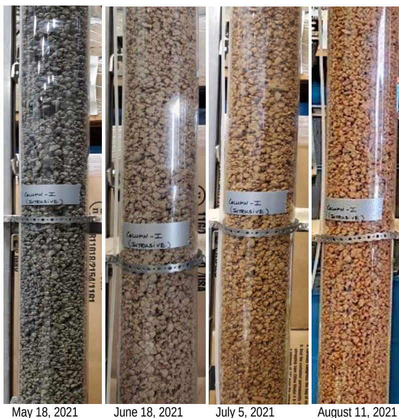
Figure 1-2: Column of Intrusive Composite Sample Under Oxidation
