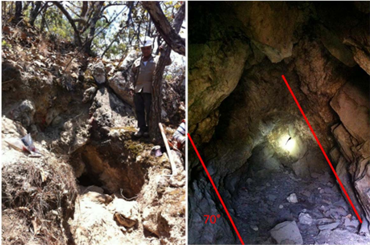
FIGURE 9.14 MINE WORKING OVER THE VISTA HERMOSA VEIN, PHOTOGRAPHS WITH WHITE AND CRYSTALLINE QUARTZ, 0.90 m WIDE VEIN
