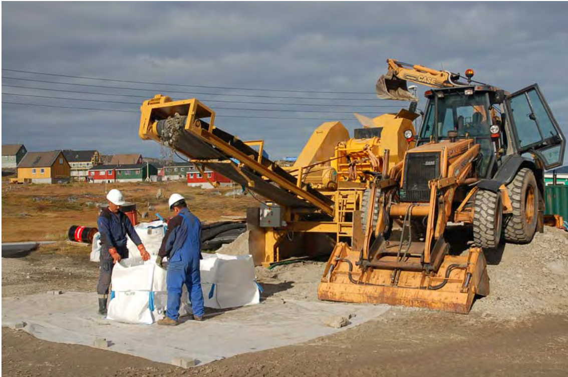
Illustration 27. Primary and secondary jaw crushing at Fiskenaasset plant – all samples contained in super sacs between 1st and 2nd crush, and after 2nd crush to wet screening.
