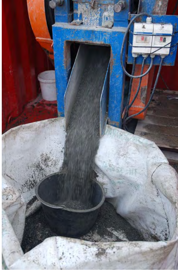
Illustration 29. Secure containment of tertiary roll crushed samples, after primary screening, and prior to final screening and jigging; progressive staged roll crushing from maximum opening of 14mm to minimum of 5mm.
