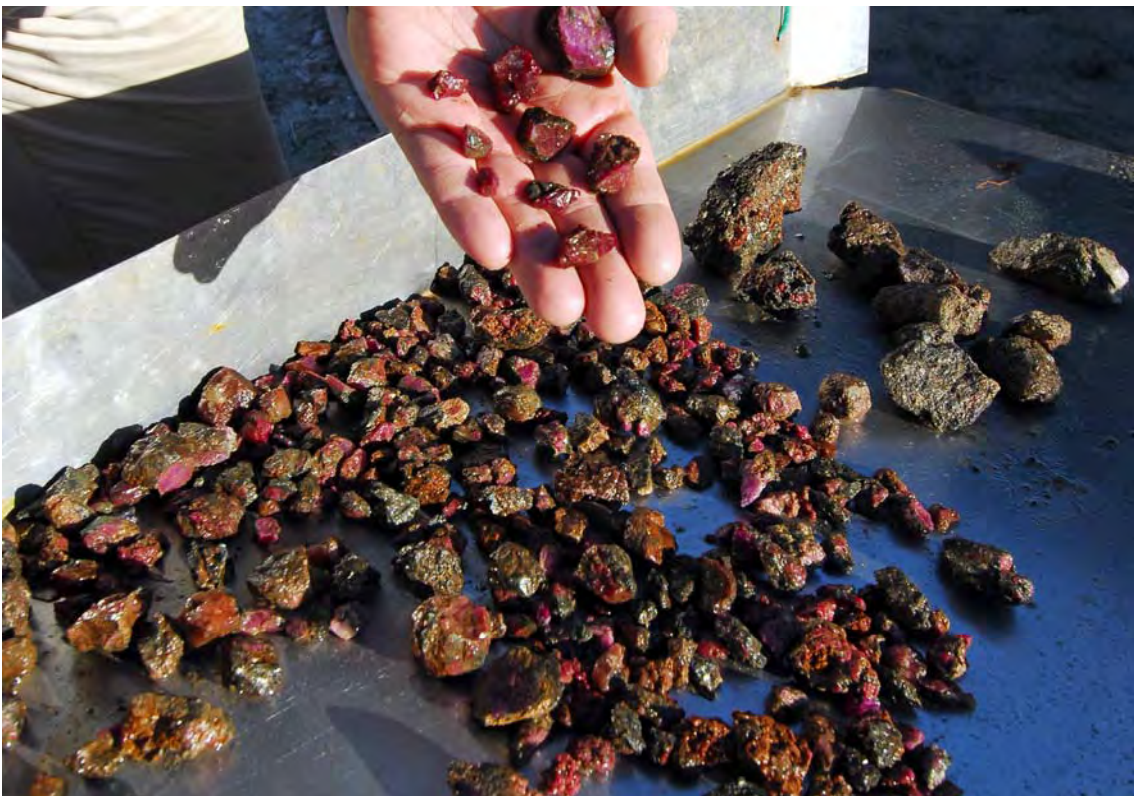
Illustration 33. Example of hand sorting of +25mm and +10mm oversize ruby and pink sapphire from 2007 Aappaluttoq soil.
