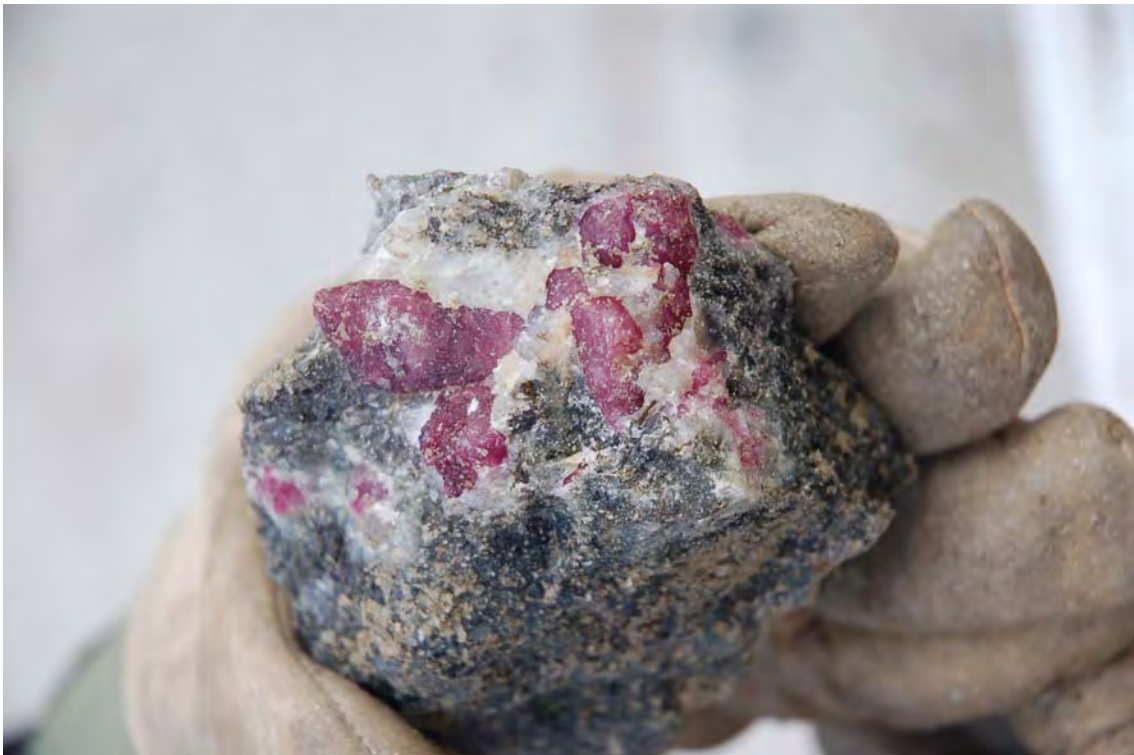
Illustration 28. Coarse-grained ruby mineralization recovered by hand cobbing during primary jaw crushing at Fiskenaasset plant.
