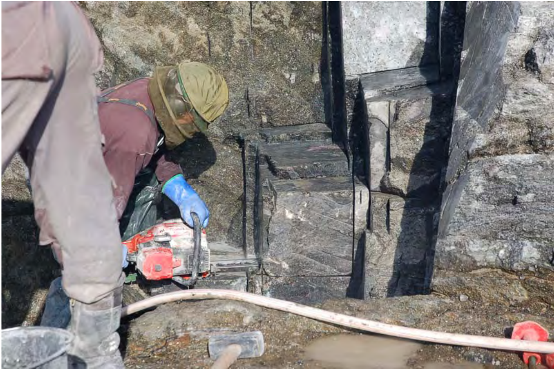
Illustration 17. Chain saw extraction of bulk samples at Aappaluttoq during both 2006 and 2007 (image from July 2007) – total approximately 55 tonnes removed by this method.
