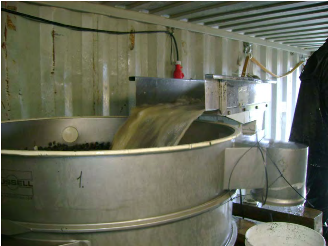
Illustration 30. Two double-deck wet washing screens with individual decks at 10mm, 6.3mm, 3.4mm and 1.7mm; -1.7mm is directed to tailings pond.
