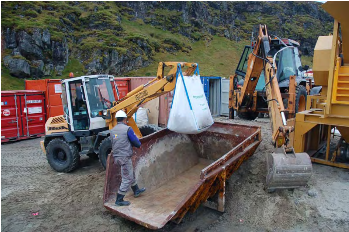
Illustration 24. Transportation of 2007 bulk samples in Fiskenaesset by loader into clean hopper for loading by backhoe into primary and secondary crusher.
