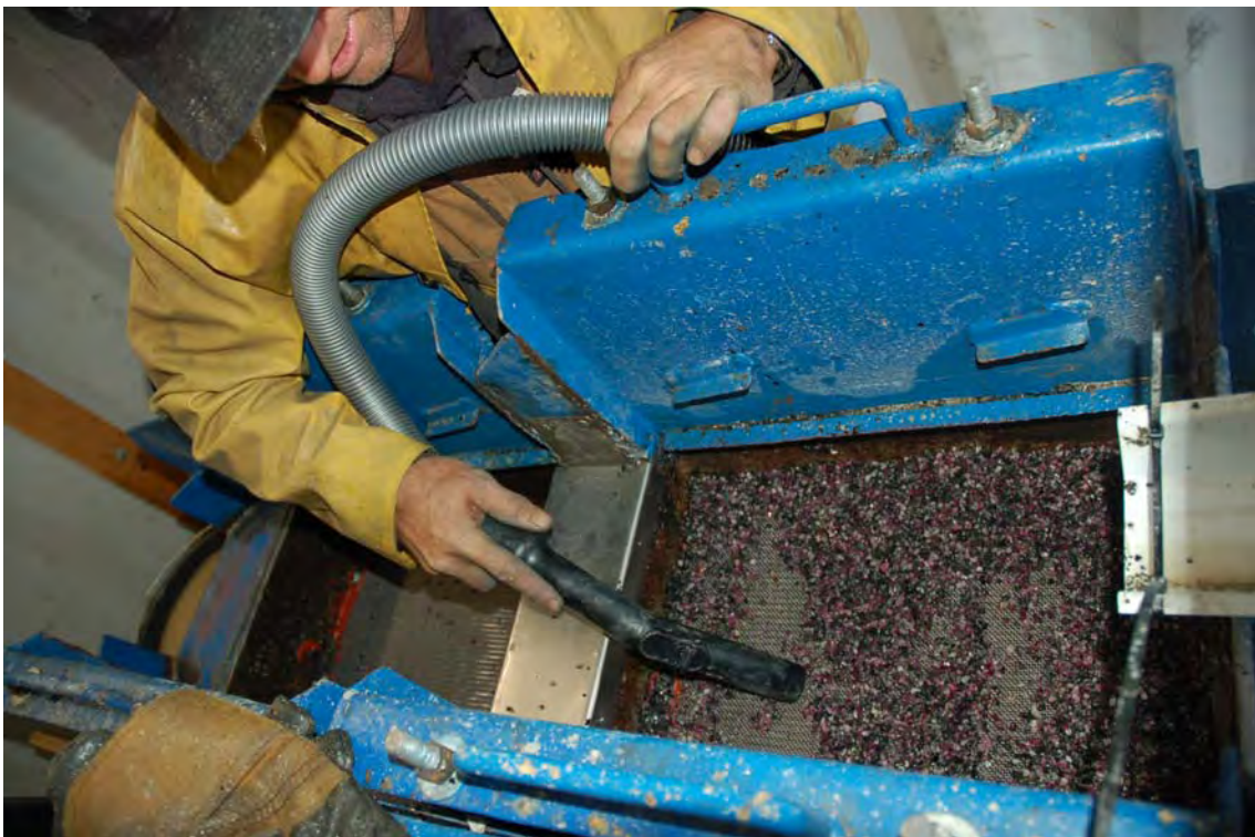
Illustration 31. Denver duplex jig with secure cleaning of concentrates by vacuum for packaging and direct hand delivery, by plant manager or project manager, to secure drying, screening and sorting facility in Fiskenaasset.
