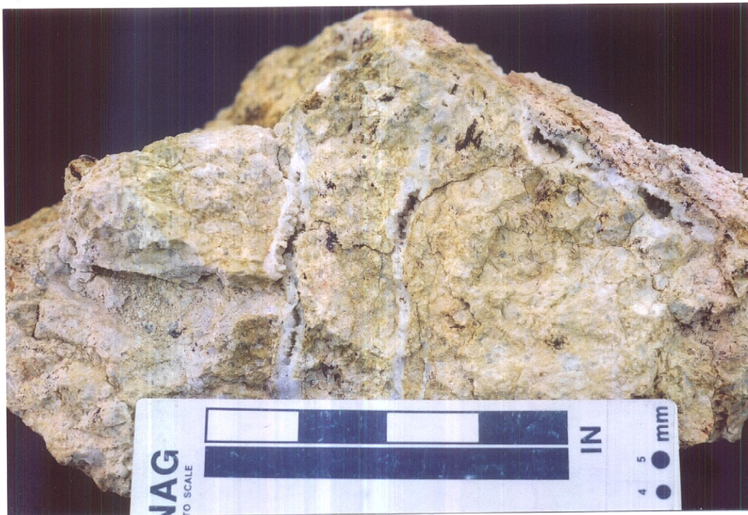
Photo 6 Hand sample exhibiting steam-heated, advanced argillic alteration (quartz-alunite [?] \pm clay) that hosts a stockwork of vuggy quartz veinlets (Arrowhead mine site).
