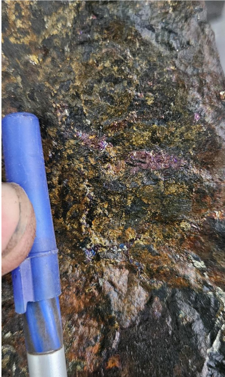
Figure 3. Chalcopyrite and bornite from grab sample SCFS-25-062 at Gimlet Target Area.
