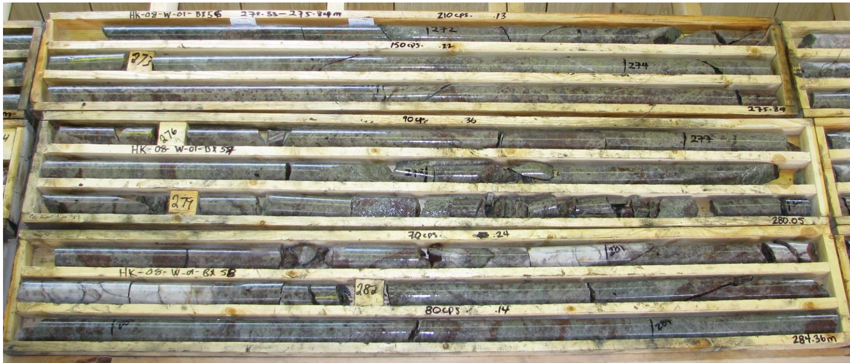
Figure 39: Core Photo of HK08-01 Showing Sericitized and Silicified Quartz Diorite
