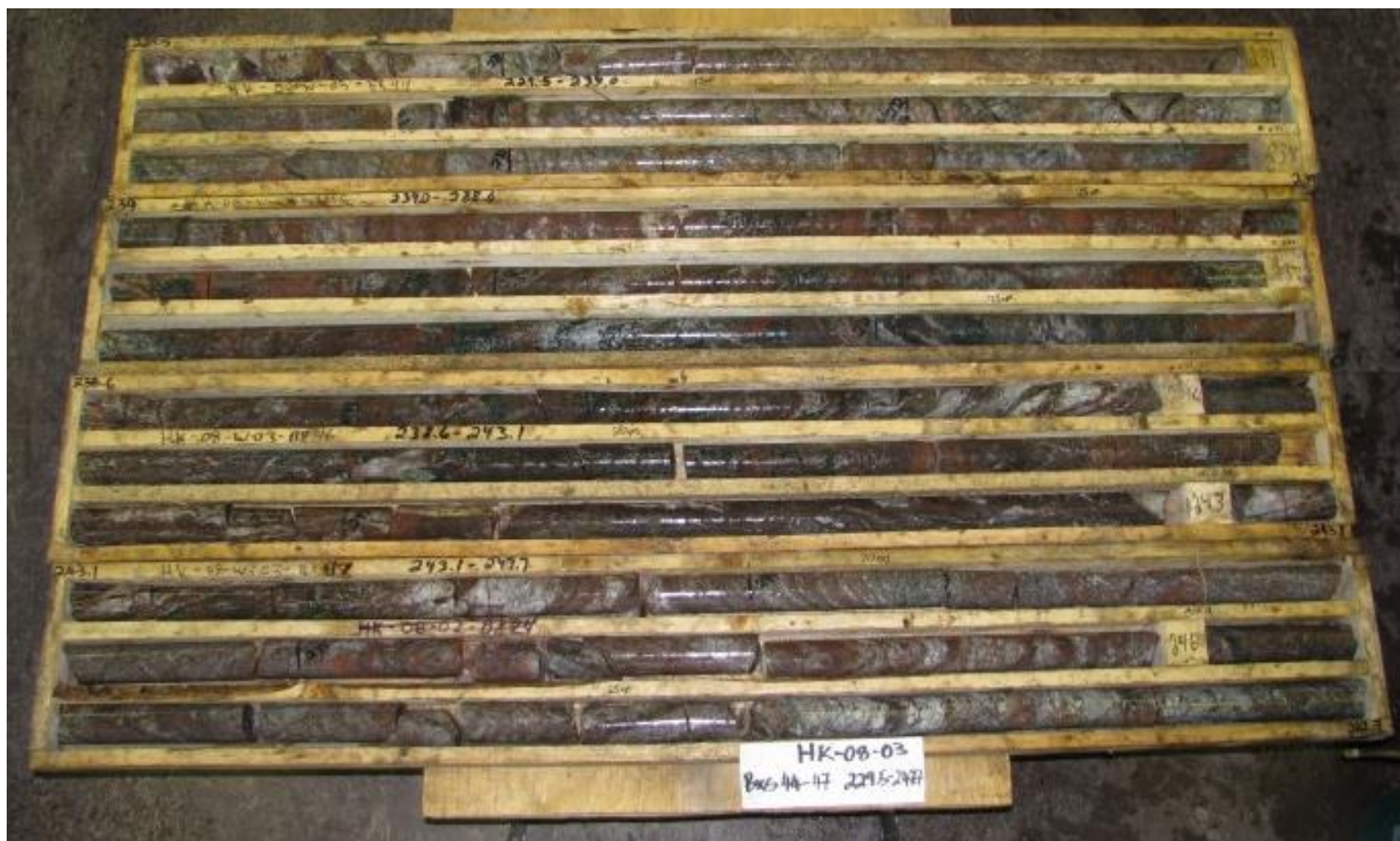
Figure 40: Core Photo of HK08-03 Showing Hematized and Silicified Diorite Gneiss
