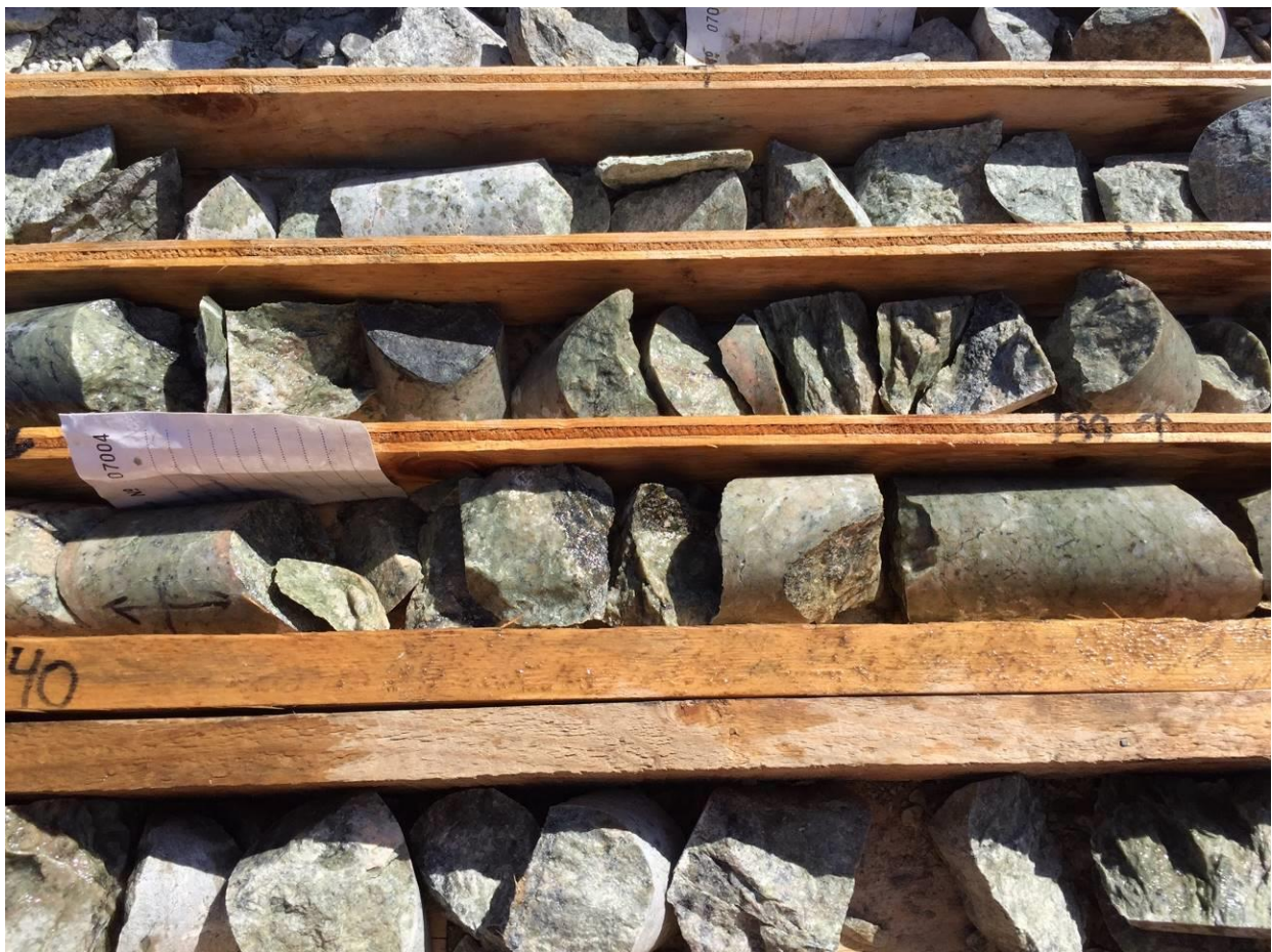
Figure 7-10 Pervasive Phyllic (sericite) Alteration, Bornite Zone, hole 114, centered at 140.0m
