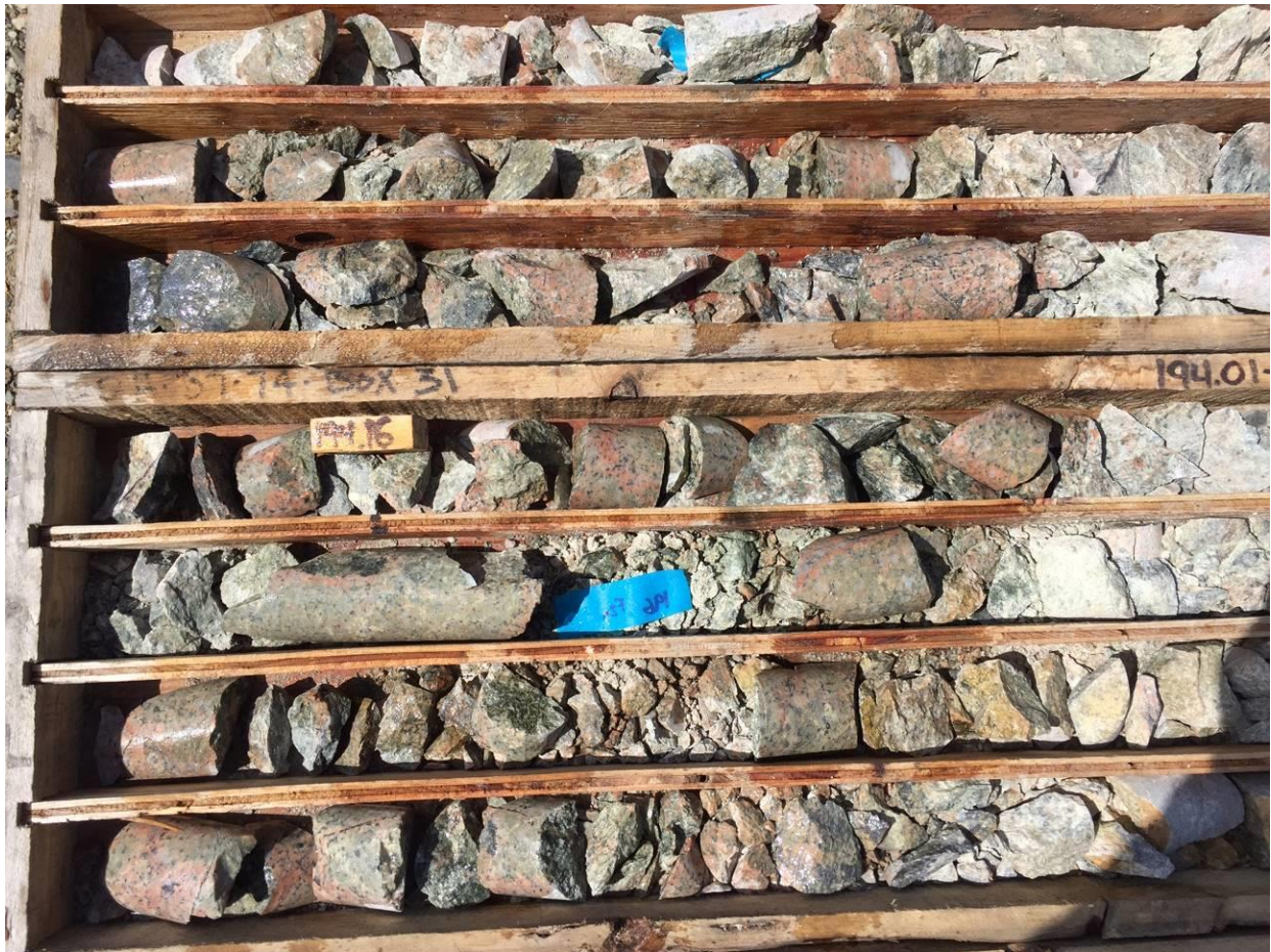
Figure 7-6 Mixed Potassic (k-feldspar) and Phyllic (sericite) Alteration, East zone, hole 107, centered at 194.0m
