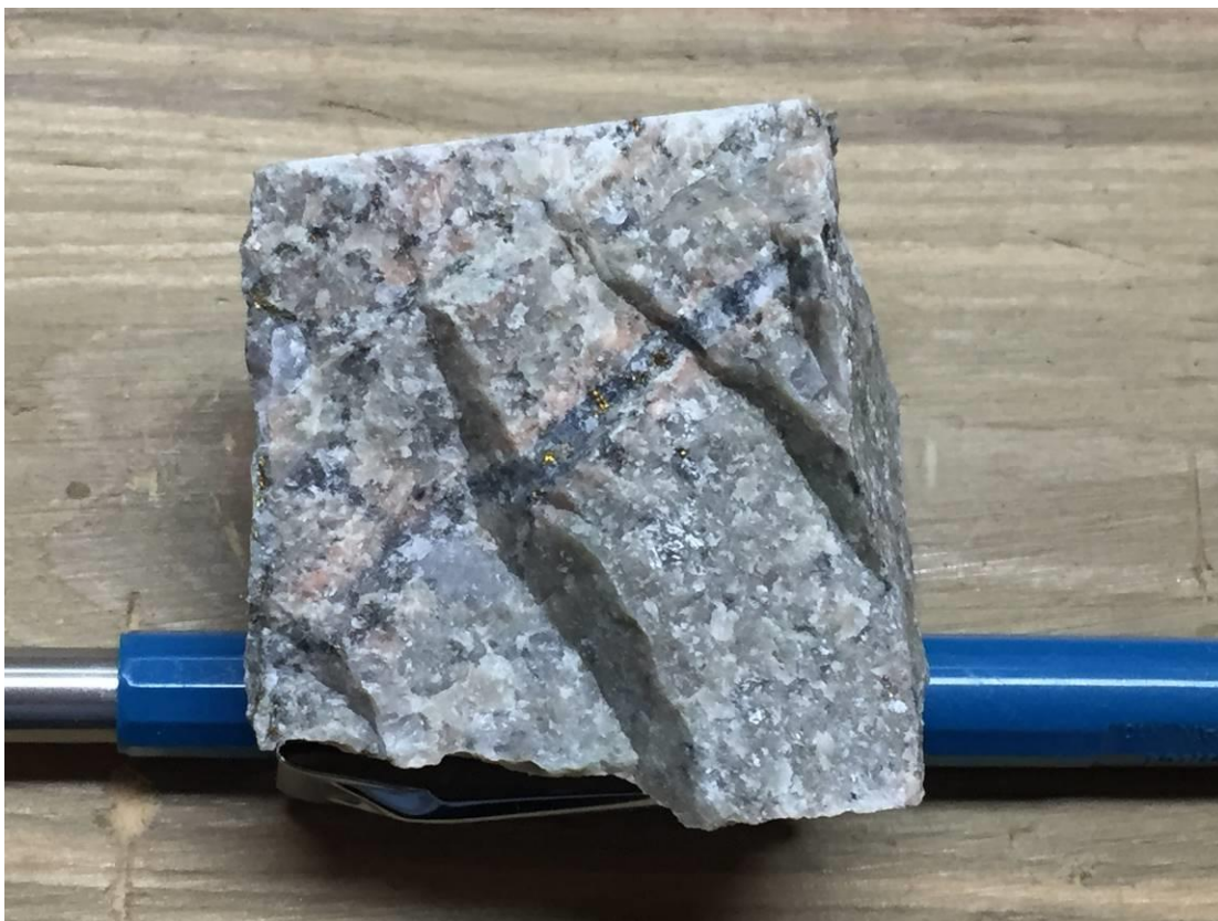
Figure 7-7 Close-up of Core Displaying two Orientations (parallel to core axis and at 30° to core axis) of Quartz-chalcopyrite+/-molybdenite veinlets, East Zone, hole 107 at 194.2m
