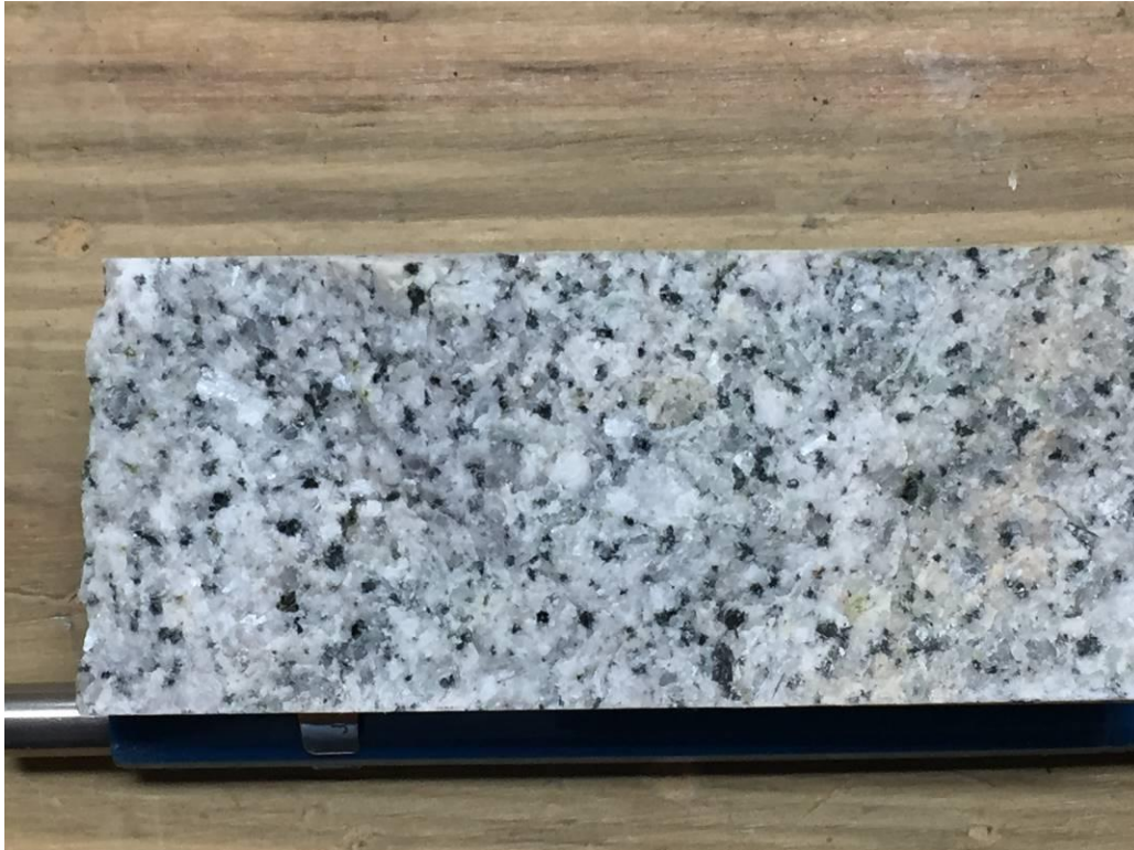
Figure 7-13 Weak Propylitic Alteration, Biotite Hornblende Granodiorite, Pass zone, hole 48 at 131.4m
