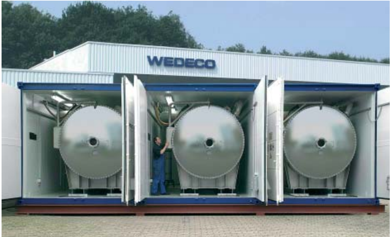
Every day three WEDECO ozone generators with a combined performance of more than 500 kilograms an hour bleach some 2,400 tonnes of cellulose per day for Votorantim Celulose Papel, one of the largest cellulose factories in Brazil
