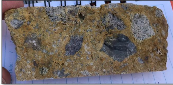
Hole CLATDH0015 – 312 m 0.05 g/t Au and 0.5 g/t Ag Quartz-jarosite-alunite low grade cap. Breccia with vuggy texture matrix of quartz with crystalline jarosite and alunite. Clast of vuggy silica and banded chalcedony (ruptured silica seal?).
