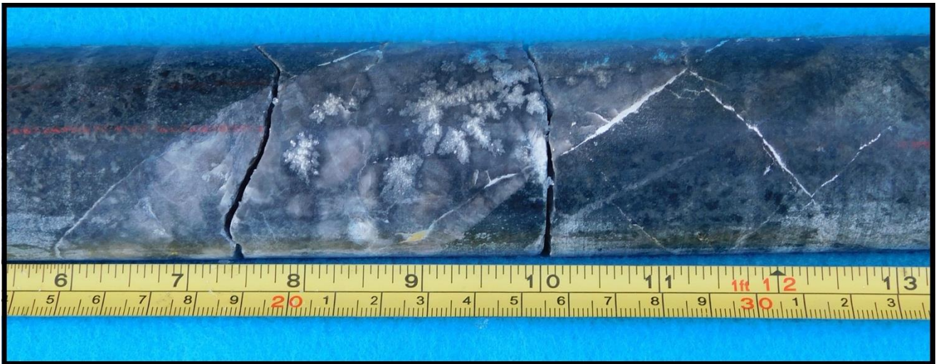
Hole CS26-129W2 at 483.2m downhole showing silver-cobalt mineralization in quartz-carbonate vein with native silver in wallrock fractures
