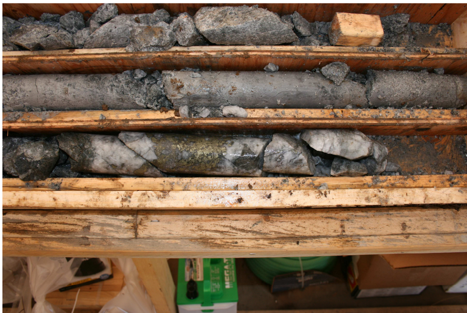
Massive chalcopyrite + arsenopyrite in quartz from MC08-05 (Sample E020404)
