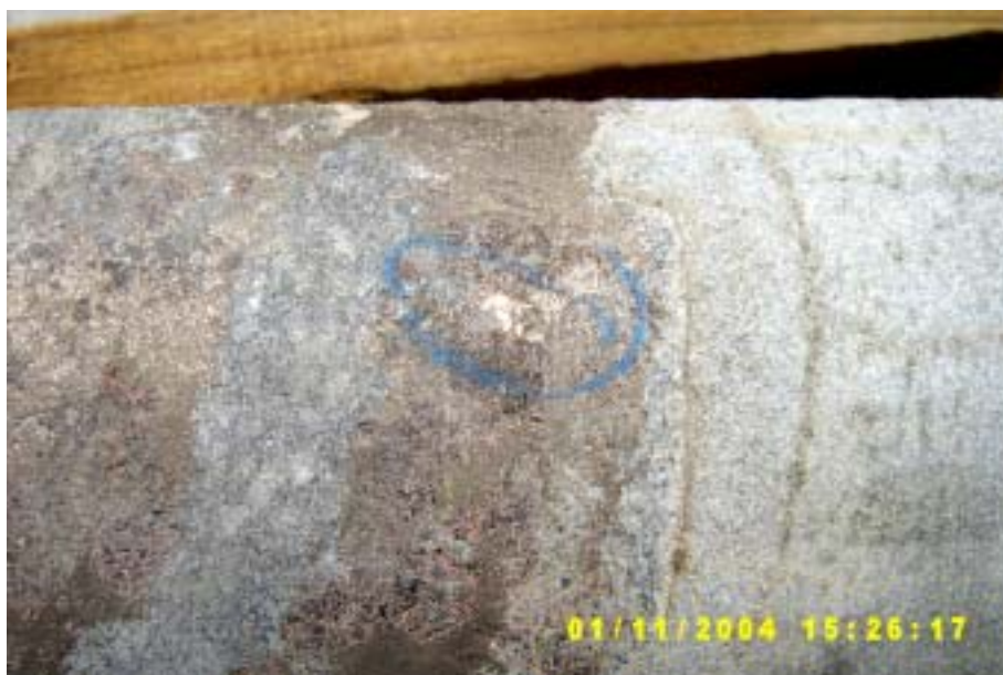
Figure 9_2 Visible gold (approximately 3mm across) in drill core – hole OT24 at 105m depth
