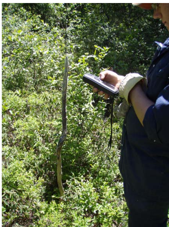
Figure 12.7 – Technician verifying the location of a historical hole by handheld GPS before spotting the new location for a planned drill hole (2010).
