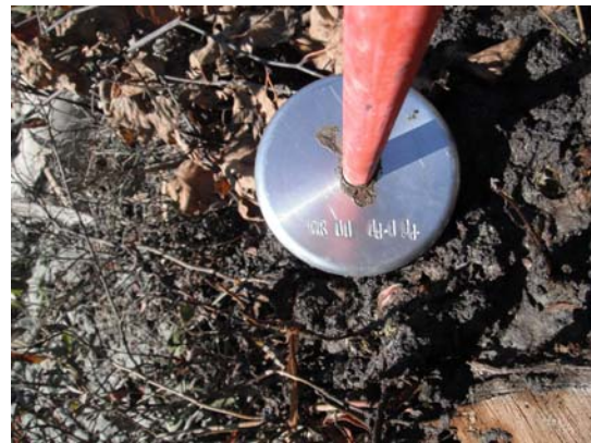
Figure 12.9 – Example of metal casing cap with red metal flag attached for hole CR-11-414, showing engraved drill hole identification number on metal cap.
