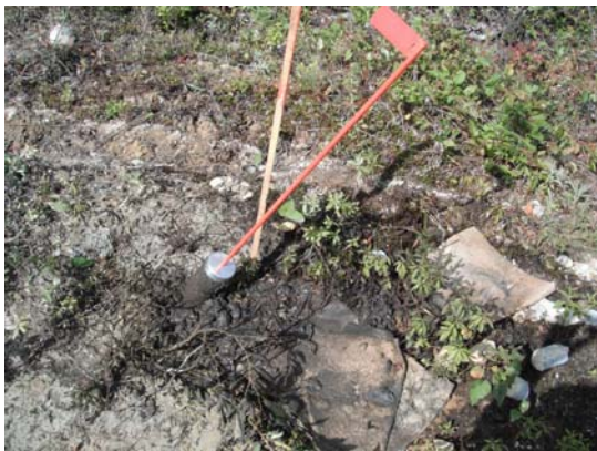
Figure 12.9 – Example of metal casing cap with red metal flag attached for hole CR-11-414, showing engraved drill hole identification number on metal cap.
