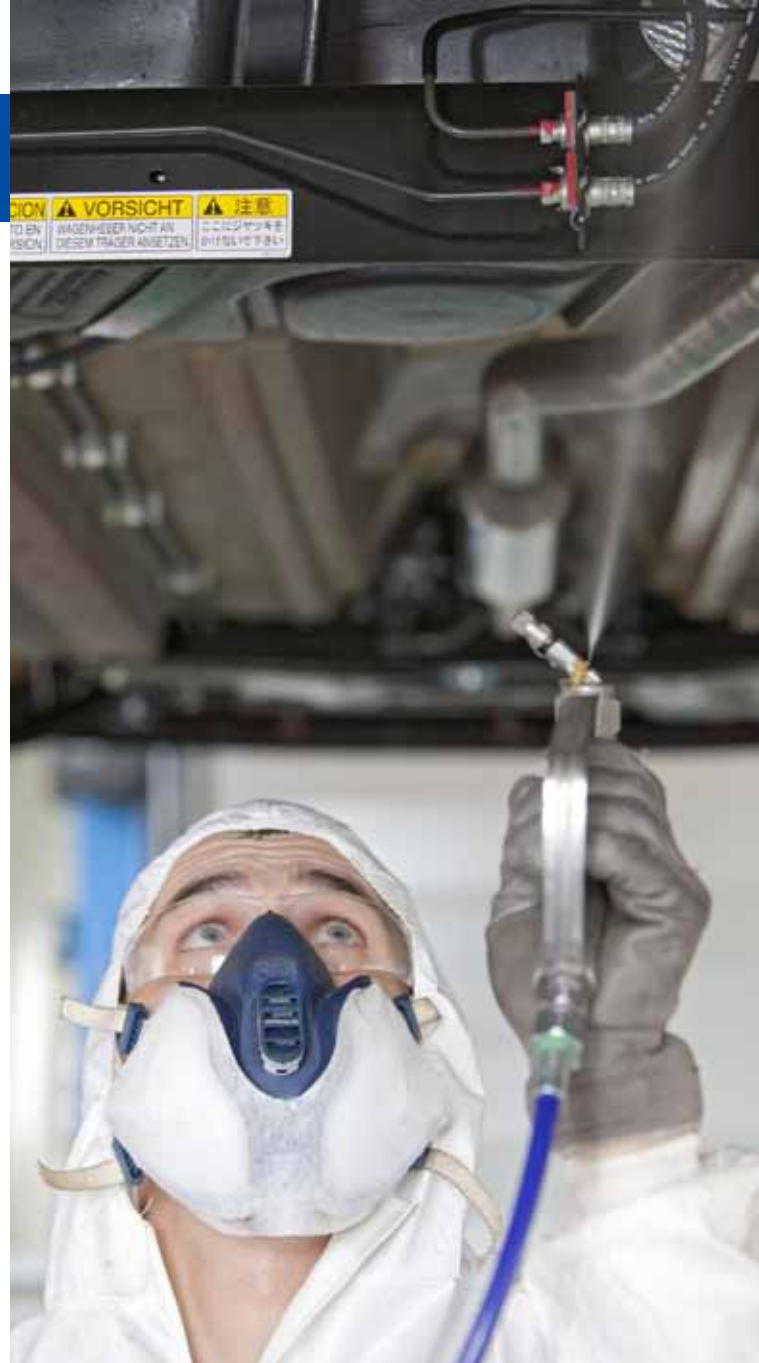
Cavity sealing work on cars at BLG AutoTec in Bremerhaven
