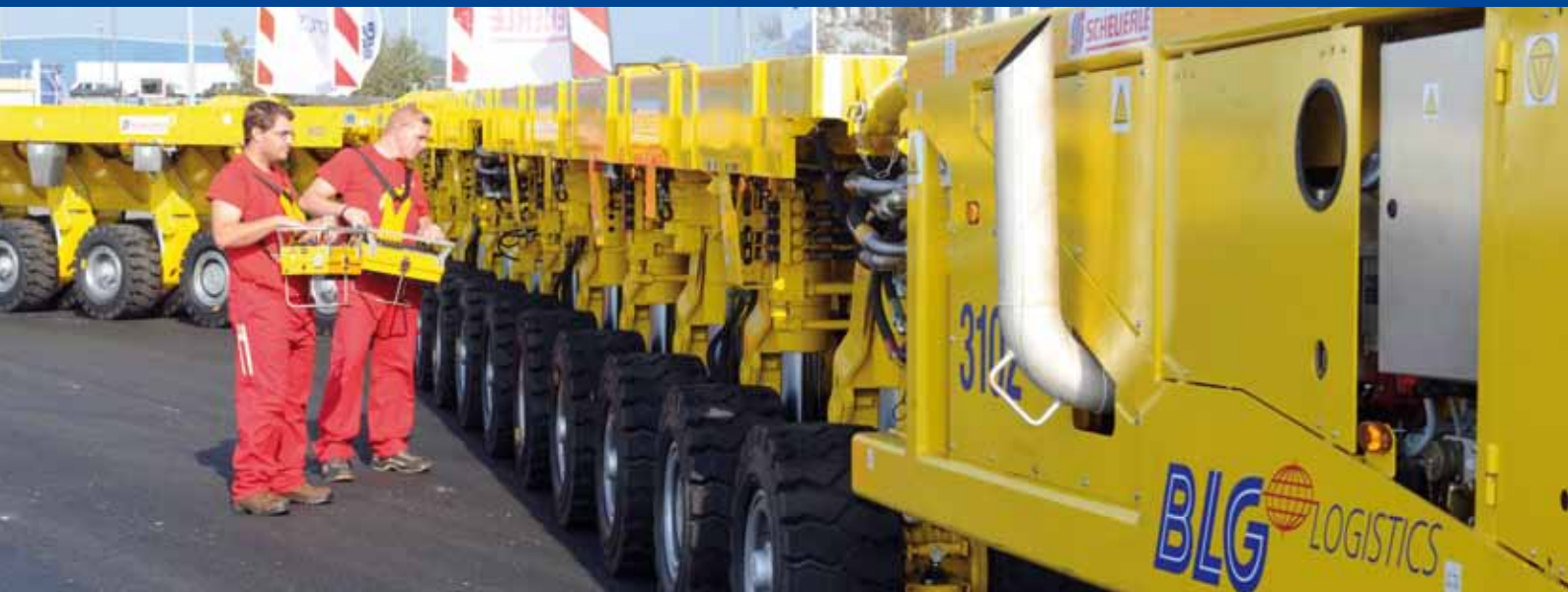
SPMT transport vehicles for heavy offshore components on ABC peninsula in Bremerhaven.
