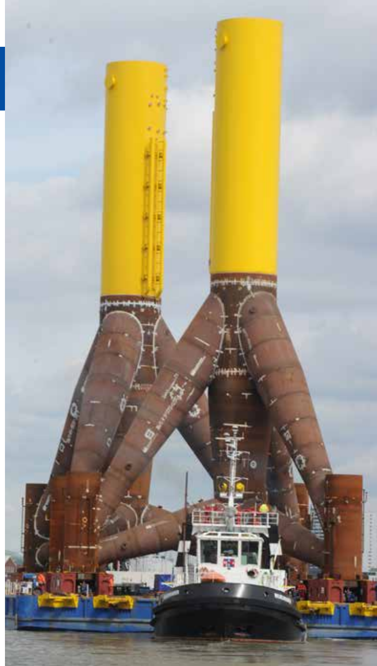
Tripod transport in Bremerhaven with the pontoon OFFSHORE BHV 1
