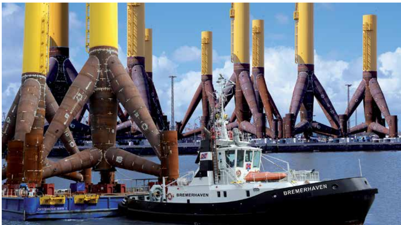
Transport and storage of tripods at BLG Offshore Terminal on ABC peninsula Bremerhaven
