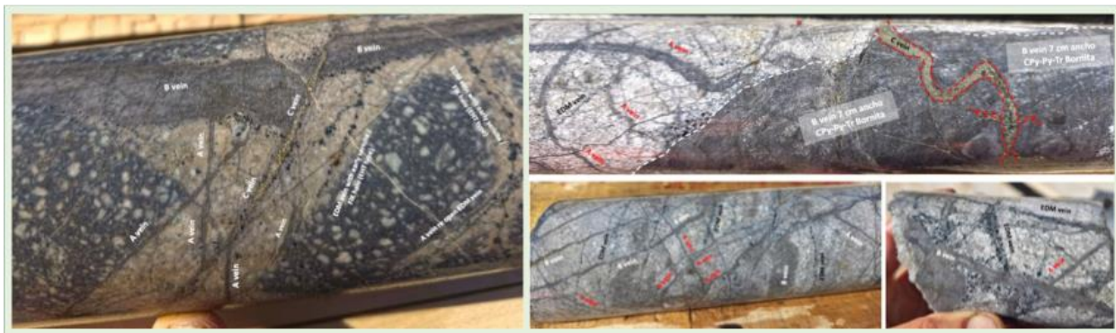
Figure 3: Mineralized vein textures in hole PIU09. Left: Dioritic porphyry with crowded veinlets. Type A veinlets cut by Type B and subsequently by Type C veins at ~543 m depth. Top right: ~7 cm wide Type B vein containing chalcopyrite-pyrite-bornite mineralization at ~557.2 m. Bottom right: Mineralized veinlets and EDM veins between ~553 m and ~560 m depth.
