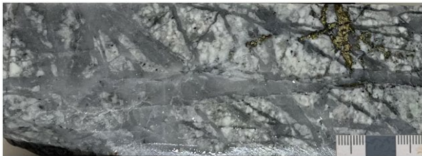
278.20m (Sample G543179: 0.51% Cu, 70ppm Mo): Porphyritic rhyolite with quartz "eyes" and weak to moderate sericitic alteration. The core exhibits A-type stockwork veinlets with traces of chalcopyrite (Cpy) and bornite (Bn), plus disseminated molybdenite (Mo) and patches of chalcopyrite (Cpy) plus hairline fracture-fill.
