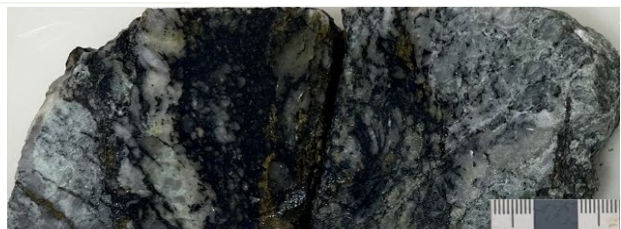
334.55m (Sample G543211: 1.64% Cu, 106ppm Mo): Porphyritic rhyolite with strong Grey-Green-Sericite (GGS) alteration. Chalcopyrite (Cpy) and bornite (Bn) occurs in fine veinlets/structures and influenced by a shear zone.
