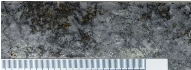
300.80m (Sample G543192: 0.97% Cu, 113ppm Mo): Hydrothermal breccia of rhyolitic composition with Grey-Green-Sericite (GGS) alteration and moderate silicification. Mineralization comprises fine A-type veinlets with traces of chalcopyrite (Cpy) and bornite (Bn) in hairline fractures and as disseminations.
