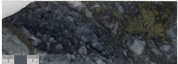
310.10m (Sample G543198: 0.43% Cu, 352ppm Mo): Rhyolitic rock with fragmental texture and sericitic alteration and moderate silicification. Pyrite (Py) and chalcopyrite (Cpy) occur in veinlets and patches, with disseminated molybdenite (Mo).
