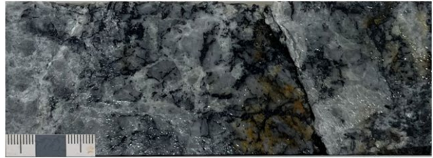
258.38m (Sample G543168: 0.87% Cu, 366ppm Mo): Porphyritic rhyolite with fragmental texture (brittle deformation) and predominant Grey-Green Sericite (GGS) alteration. Bornite (Bn), chalcopyrite (Cpy), and molybdenite (Mo) mineralization occurs as hairline veinlets (fracture fill) and disseminations.
