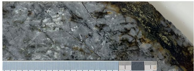
284m (Sample G543183: 1.09% Cu, 71ppm Mo): Magmatic breccia of rhyolitic composition with Grey-Green-Sericite (GGS) alteration and moderate silicification. A-type veinlets host traces of chalcopyrite (Cpy) and bornite (Bn), present as hairline fractures and fine veinlets with minor molybdenite (Mo).
