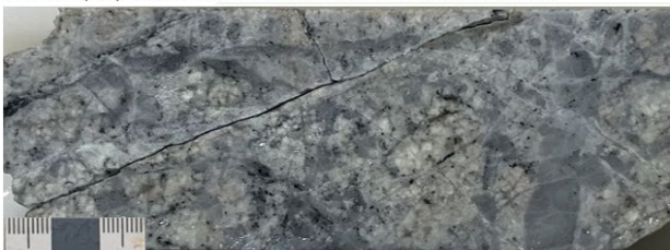
323.20m (Sample G543204: 0.29% Cu, 38ppm Mo): Porphyritic rhyolite with fragmental texture, quartz "eyes," medium to coarse-grained crowded texture, and sericitic alteration overprinting potassic alteration. Mineralization comprises early A-B type veinlets with traces of chalcopyrite (Cpy) and molybdenite (Mo), with bornite (Bn) and chalcopyrite (Cpy) as disseminations.
