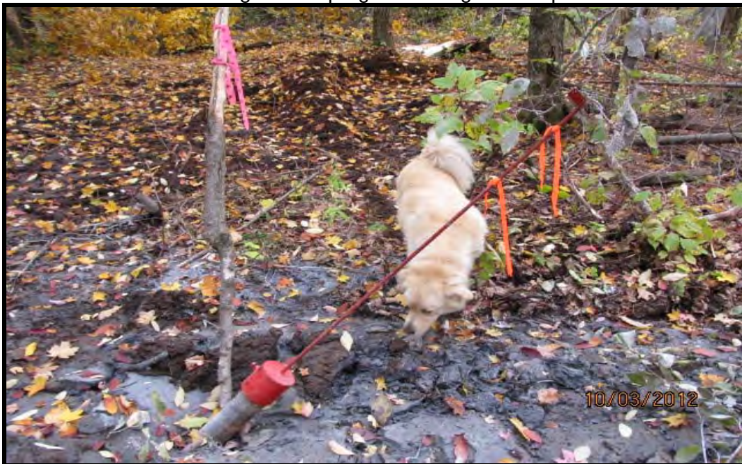
Photo 2: Drill hole casing of a 2012 exploratory drill hole.
