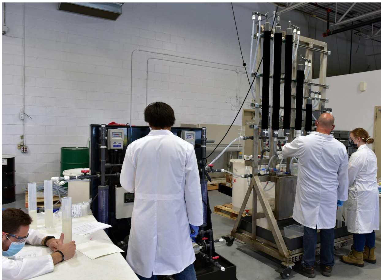
Image 1: KPM technicians operating the RapidSX™ test platform during REE extraction-rate testing. The test was conducted on June 28, 2021, at IMC's RapidSX Commercialization Development Facility in Kingston, Ontario. Photo: Innovation Metals Corp.
