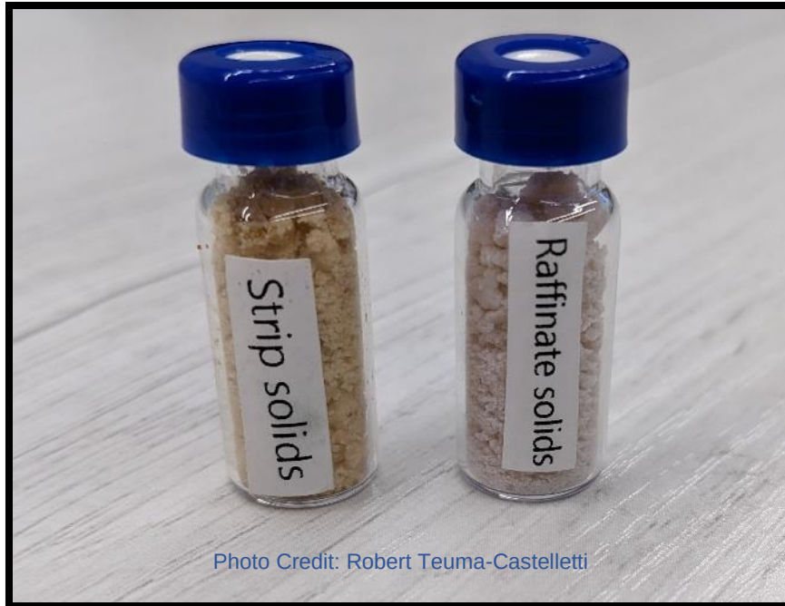
Figure 1 - Separated Heavy REE (from Ionic Clay Sourced Material) Sample Products from the RapidSX™ Demo Plant Commissioning Trials
