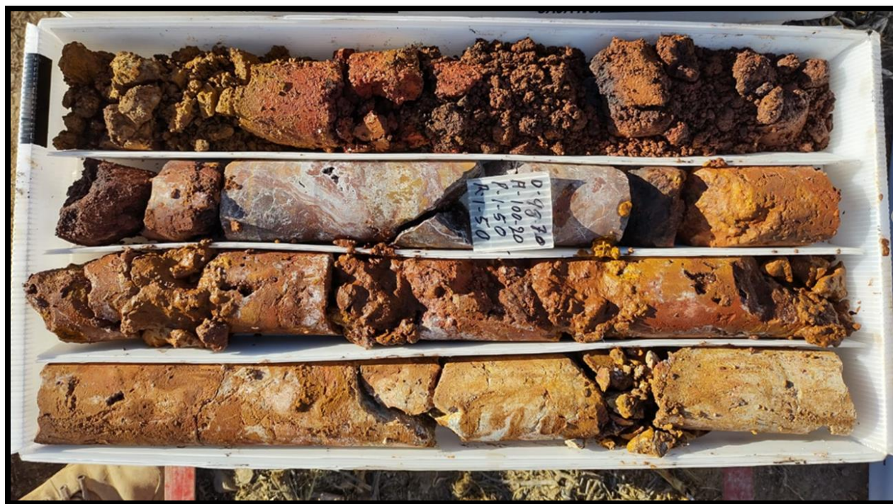
“Core from hole SJ 021, exhibits evident mineralization with supergenic effects, which is composed of secondary hydroxides and clays.” – Dr. Rocha-Rocha
