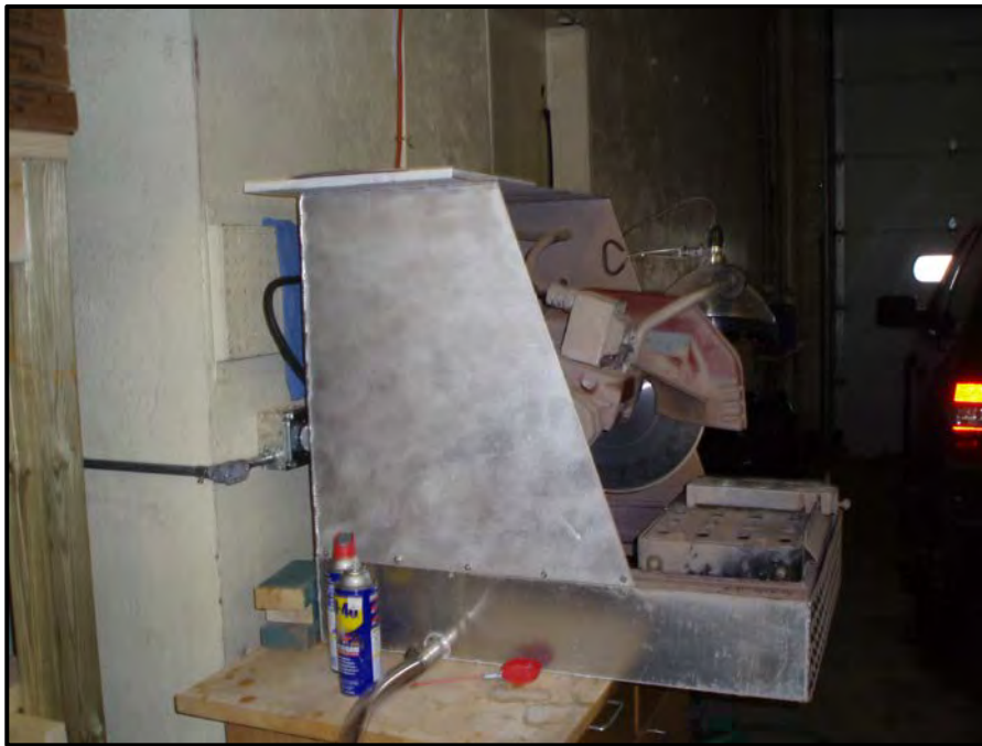
Figure 10.5: Core saw station
