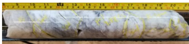
Figure 2.1 – Photo of drill core displaying pollucite from West Joe at the Company's Case Lake Property, Ontario, Canada (CNW Group/POWER METALS CORP)
