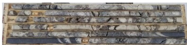
Figure 2.2 – Photo of drill core displaying pollucite from West Joe at the Company's Case Lake Property, Ontario, Canada (CNW Group/POWER METALS CORP)
